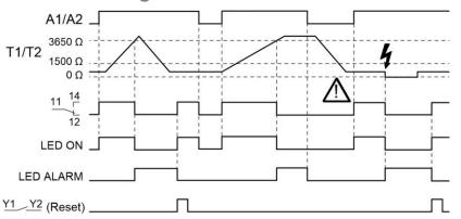
Caution! The device switches on automatically after a supply voltage dip.
