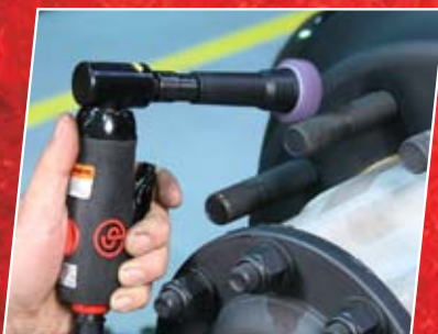
Clean the drum and studs with a CP7562 Mini Angle Grinder
