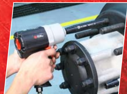
Tighten the nuts with a CP7749 1/2" Impact Wrench
