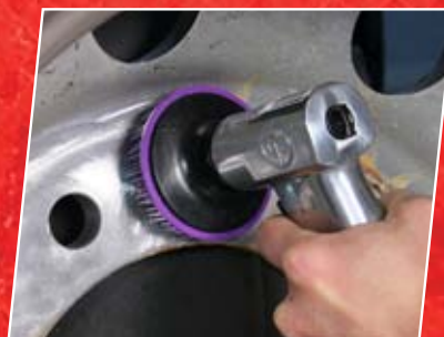
Clean the wheel with a CP7202 Mini Disc Sander
