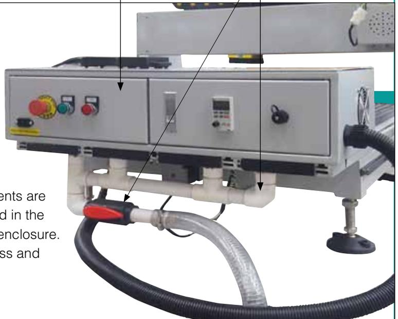
All the electrical components are housed, wired and tagged in the HD-II Tabletop electrical enclosure. This allows for easy access and service when needed.
