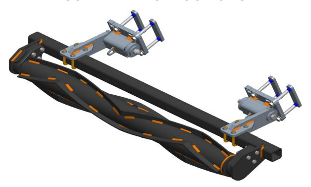
**Step 1**: Attach the 5000-167 torsion mount bracket to the frame using 4) M16 X 110 flange head bolts & 2) 5000-420 clamp straps. Thread the bolts into the clamp straps by hand & tighten to torque specifications.
