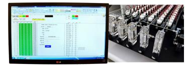
Following each critical operation in the assembly process, every sensor is tested to confirm signal output using equipment traceable to calibration certificates.
