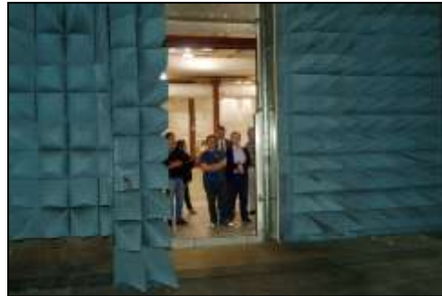
Visitors are shown one of the doors to the main test chamber in the Electromagnetic Vulnerability Assessment Facility. The main chamber which is over 100 feet long can be used for experiments with everything from computer networks to tanks and small aircraft. (Photo by Drew Hamilton)
