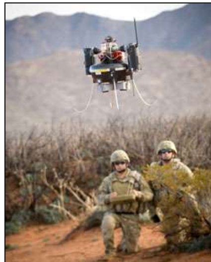
Soldiers control the Class I unmanned aerial vehicle (UAV) at White Sands Missile Range. The system is designed to provide the soldier with reconnaissance, surveillance and target acquisition. (U.S. Army PEO-I (BCT) photo.)
