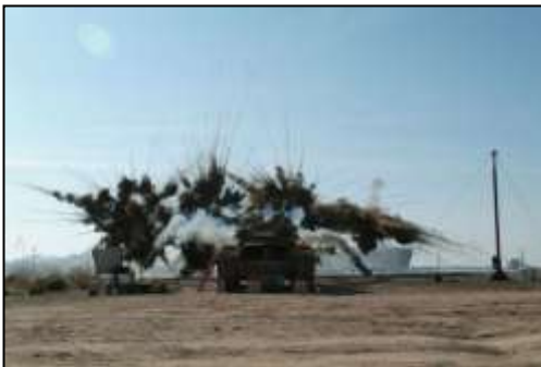
A 4-round half salvo of GALIX 13 grenades is launched from the Center for Countermeasures' M-60 tank during testing.
