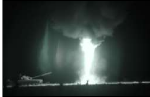
The Center for Countermeasures tests a flamethrower during nighttime testing; the flamethrower acts as a countermeasure to protect the tank from attack.
