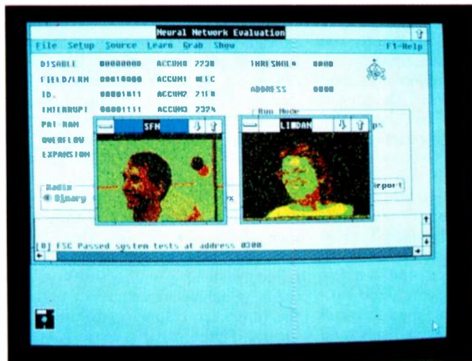
Fig. 5. Testing pattern matching ability with video picture material. The development board could happily sort out pictures with up to 10% added noise superimposed on the signal.
