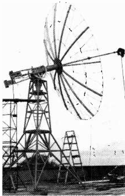
The 20ft paraboloid with helical antenna used at the University College Dublin station.
