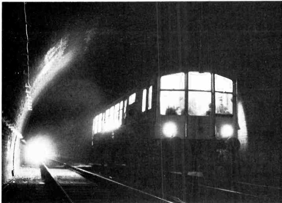
British Rail's mobile radio laboratory, test coach Iris, which has been equipped by the Research & Development Division to carry out radio system survey work anywhere on the network. Its first task was to evaluate the performance of a possible system of track-to-train
