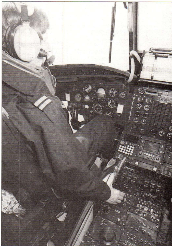
Cockpit of a modern helicopter. The radio equipment is just below the pilot's hand, with an illuminated frequency indicator panel. This could be v.h.f. or in the case of a military aircraft u.h.f.
