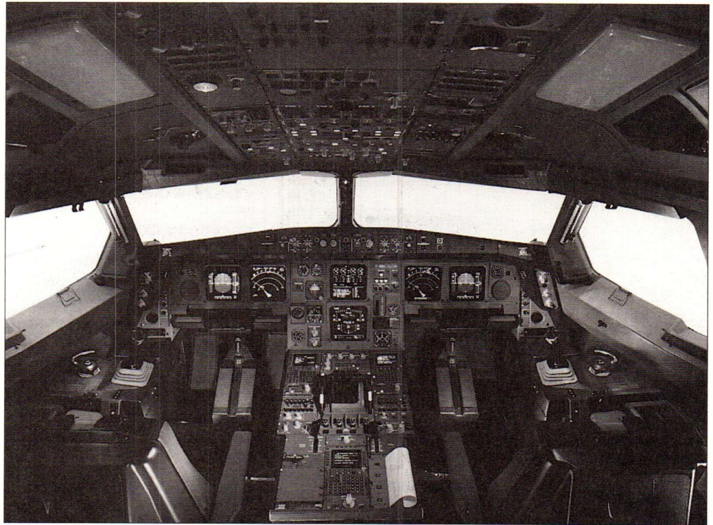
The exact locations of the v.h.f. and h.f. sets vary from aircraft to aircraft but in this case they are contained between the pilot and co-pilot's positions - the horizontal panel. There are in this case two v.h.f. sets and one h.f., the later being just above the fax output, to the bottom right hand of the console.
