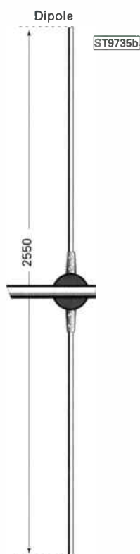
DIAGRAM 1: Dimensions for a simple dipole antenna suitable for Sporadic-E reception.
