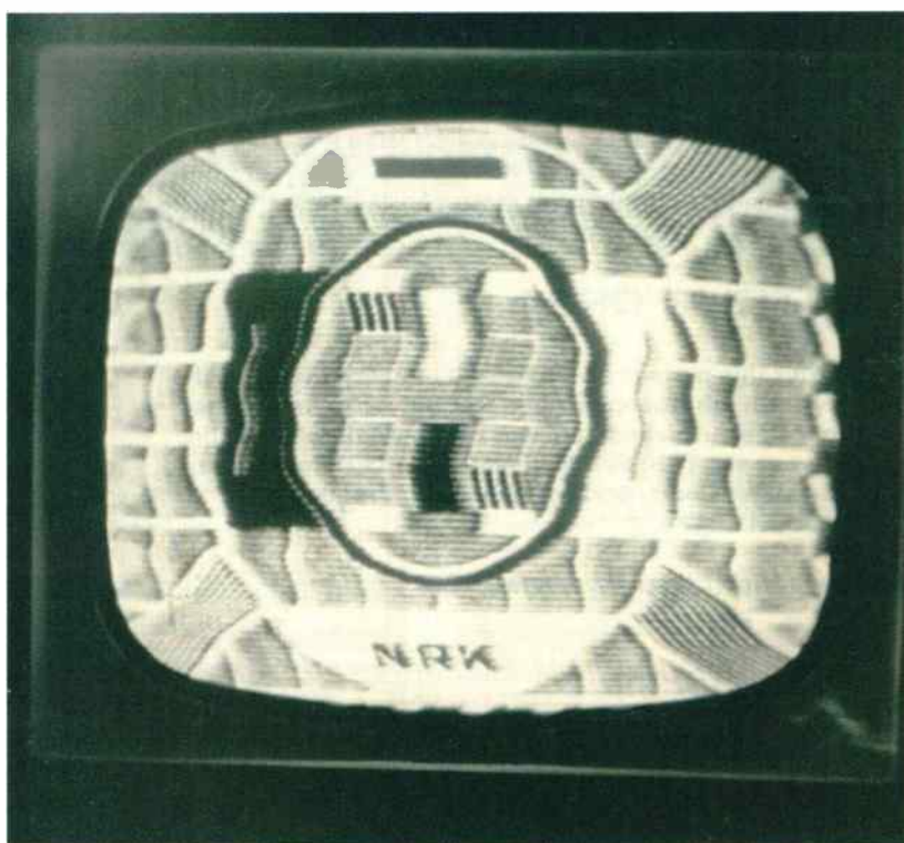
Fig.1: Test Card 'G' from Norway suffering Sporadic-E distortion, received on an indoor dipole feeding a modified Bush TV53 405-line TV receiver dating back to the late Fifties.
