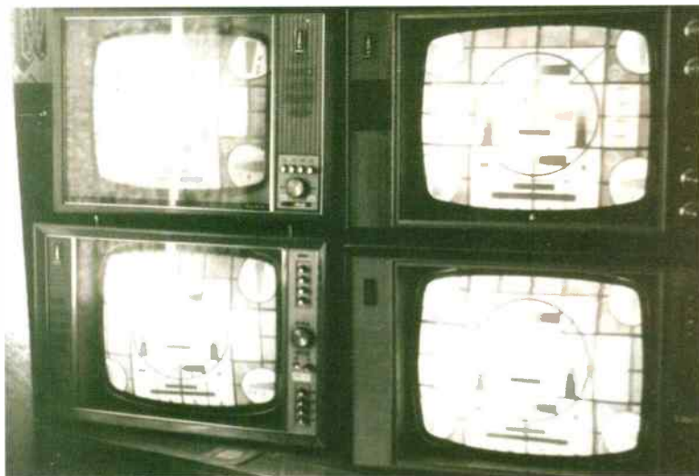
Fig. 6: A bank of 'hotted-up' Bush dual-standard receivers, each equipped with varicap tuners, capable of displaying four different channels.
