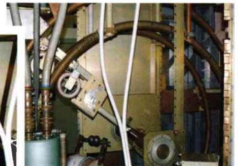
● The power amplifier tuning mechanism. Control is automated for rapid band changing.
