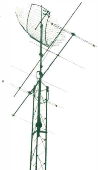
Fig. 13: An ambitious antenna system comprising separate multi-element beams covering Bands I, II and III. The top antenna is an imported 'deep fringe' parabolic u.h.f. array with a diameter of around two metres!
