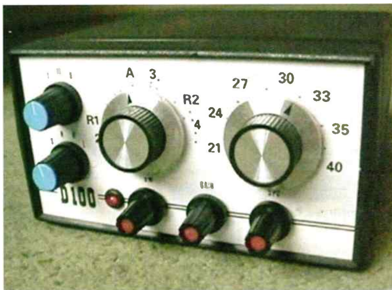
Fig.7: The D-100 external tuning system with its variable vision i.f. bandwidth.
