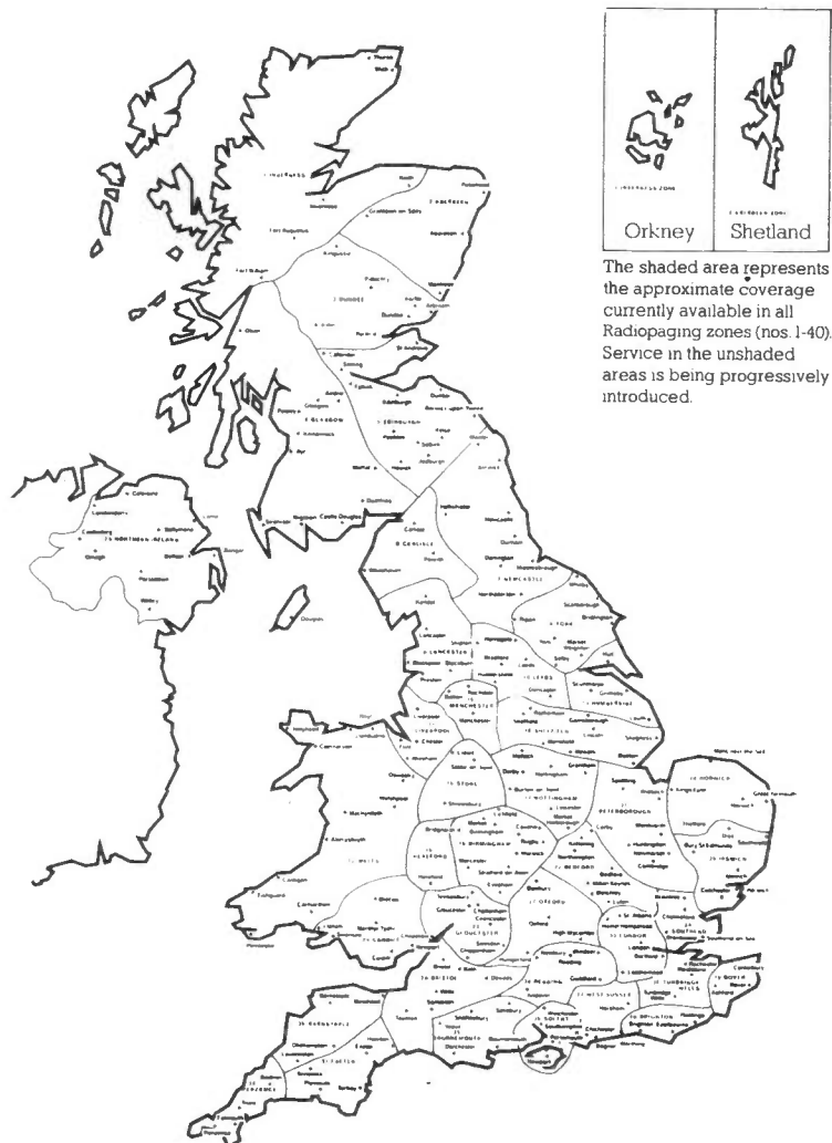
BT's national radio paging network on 153MHz is divided into 40 zones and covers 95% of the population
