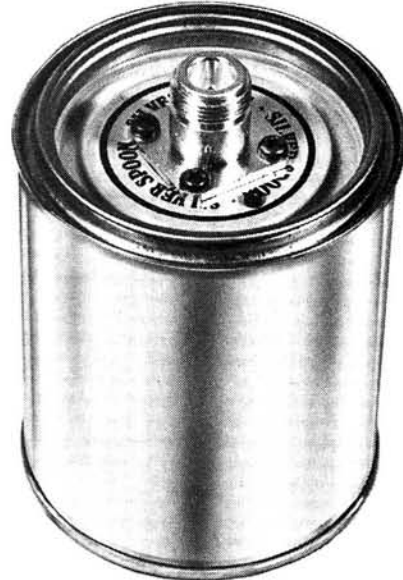
A small syrup tin is a convenient source of a box for the dummy load
