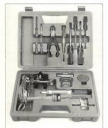
A small number of good quality tools, perhaps in a purpose built case, as in this 'Student' Tool Kit' from Maplin Electronics, can provide most of your needs. tools. Non metallic ones are essential for adjusting variable inductors.
