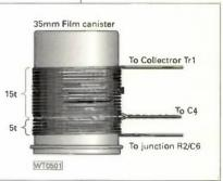
Fig. 5: Coil winding details of L1 (see text for other winding details).
