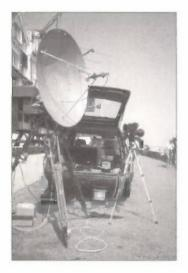
Gunn diodes make very simple and cost effective power sources for 3cm. Feed a 10mW Gunn diode into a small ex-satellite dish with a typical gain of 24dB and you achieve an effective radiated power of about 4W!
