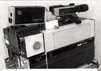
Typical ATV cameras. A monochrome ex-industrial and old domestic colour camera sit on a heavy EMI 2001 ex-broadcast studio model.
