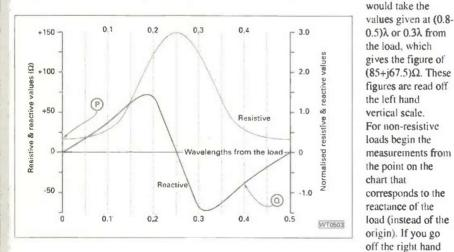
Fig. 2: The graph of the impedance variations along a line for an s.w.r. of 3:1. When no line loss is assumed, the pattern is repeated every half wavelength.
