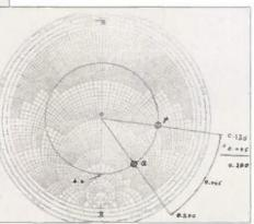
impedance  $(1.65+j1.9)\Omega$ . Multiplying this value by 50 gives the actual impedance  $(82.5+j95)\Omega$ . The input impedance of the line is therefore  $82.5\Omega$  resistive in series with 95 $\Omega$  inductive reactance.
