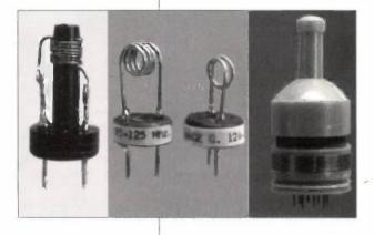
Fig. 1: Coils in various stages of construction.
