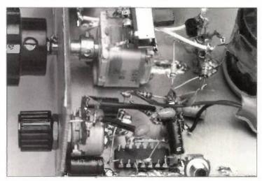
transistor Tr1 is a Hartley Oscillator where C4 is the feedback capacitor to a tapped coil L1.
