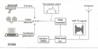
amplitude modulation (a.m.) and the picture frequencies should be limited, with a filter, to 3MHz and no colour. You may already have nearly enough kit to transmit and receive an ATV picture on the u.h.f. band.
