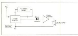
Fig. 2: Adding a tuned regenerative r.f. amplifier and an audio amplifier all increase the signal to more audible levels.
