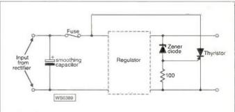
Fig. 3: A simple over voltage protection circuit.
