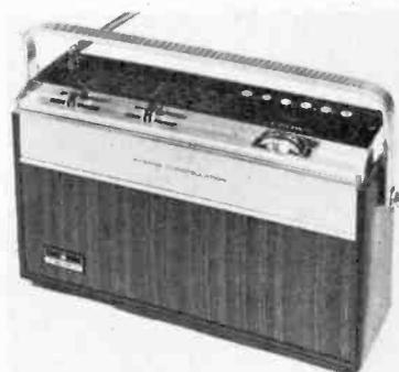
Crown TRF-2900L 4-band portable (f.m., m.w., l.w., and 49m. bandspread) Ten transistors. Price is £44 15s. inc. tax.
