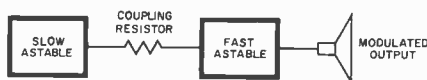
Fig. 6. A "warbling" modulated output can be obtained by interconnecting two astable square wave generators as shown here. The input connection to the second astable is made at the base of TR1 (Fig. 5 above)
