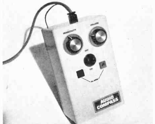
The control box of the Audio Compass, this is fitted with three suction pads for mounting purposes
