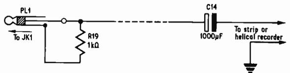
Fig. 18. Circuit for feeding output from pen amplifier into an advanced recorder
