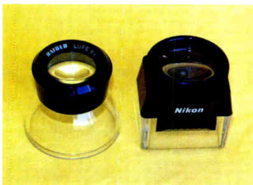
Fig.2. Checking a circuit board with a magnifying glass can highlight many soldering problems
