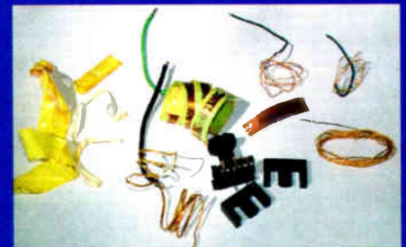
. . . allowing fairly easy disassembly. Make sure the ferrites and bobbin are very clean before going any further. Don't worry about the wire – you won't be using any of that.
