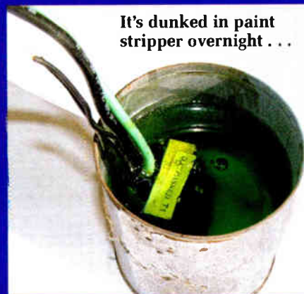
. . . allowing fairly easy disassembly. Make sure the ferrites and bobbin are very clean before going any further. Don't worry about the wire – you won't be using any of that.
