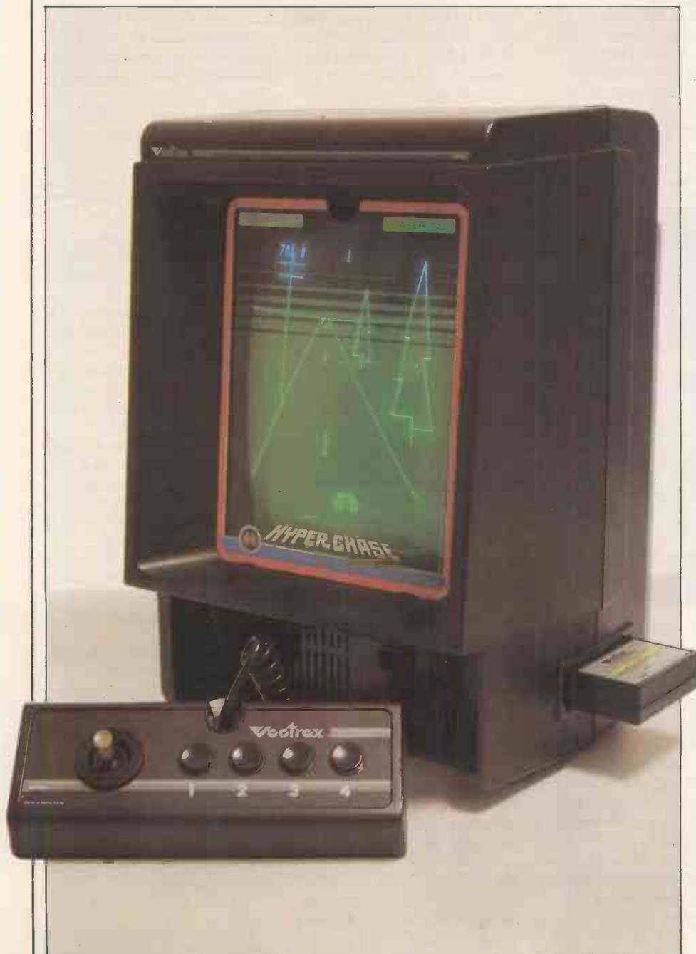
The Vectrex uses Vector graphics with three dimensional rotation and zoom.
