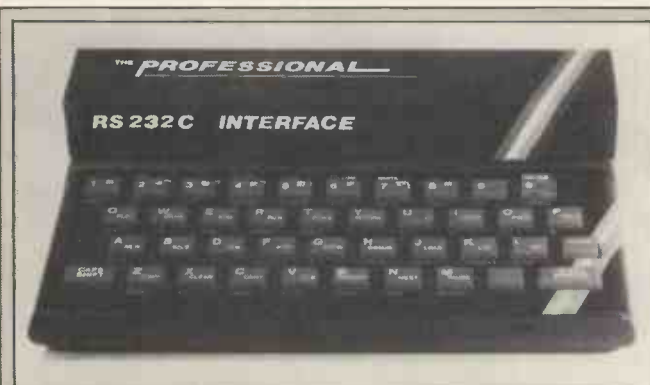
This is a Spectrum: the box on the back says it is an RS232C interface, and that is what it is. It will let you connect your machine to a printer or to a modem or to another computer (up to eight other devices, in fact).
