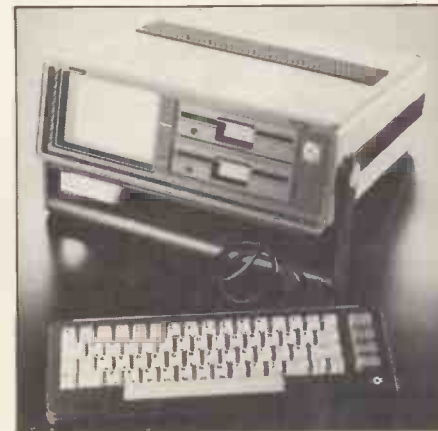
Commodore's Executive 64 uses a 6510 CPU and has Basic stored in ROM.
