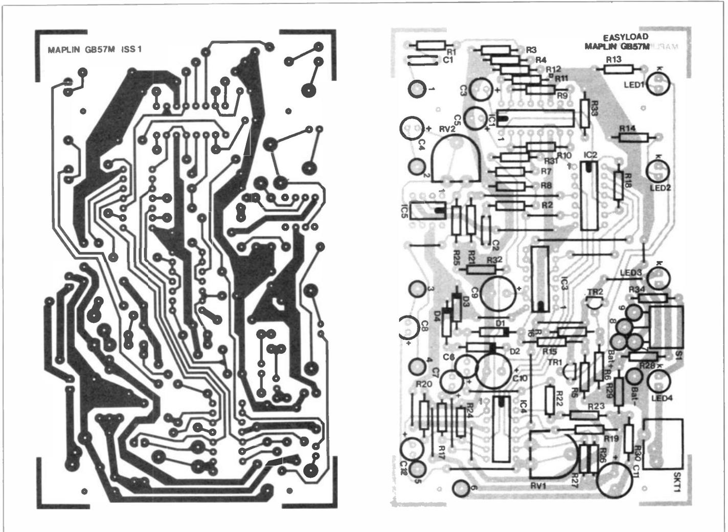
Figure 2. PCB Layout and overlay
