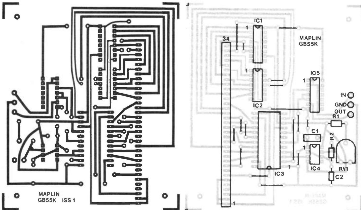
Figure 2. PCB layout and overlay
