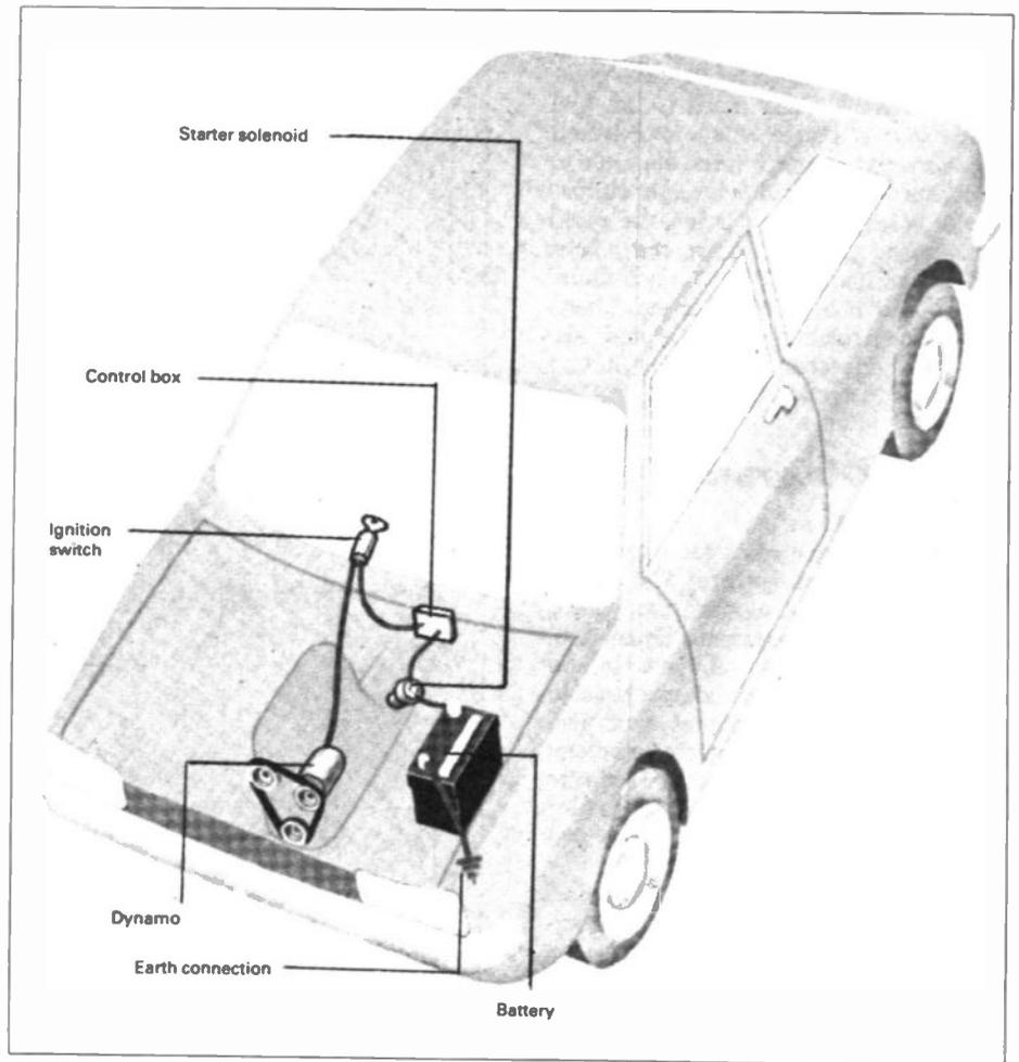
Figure 1.2. The battery charging circuit
