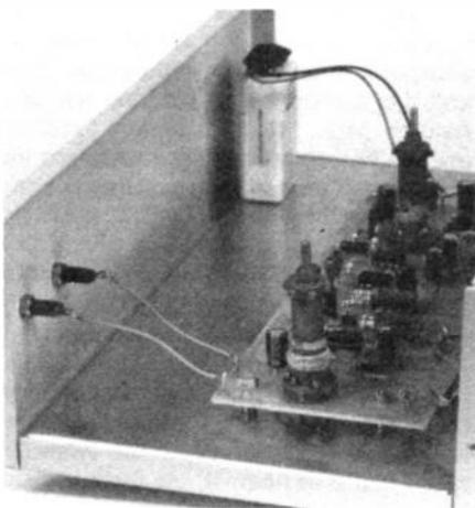
oscillator uses TR4 as a source follower stage with frequency selective positive feedback provided by T2. In order to obtain a large enough capacitance swing using BA102 varicap diodes. It is necessary to use two of these wired in parallel (D2 and D3). This permits coverage of the full 3.5 to 4.0MHz band.
