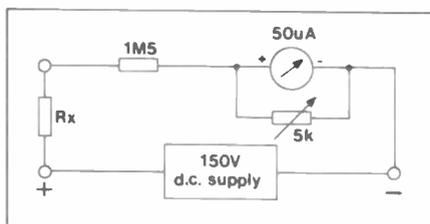
Figure 4. An insulation tester.
