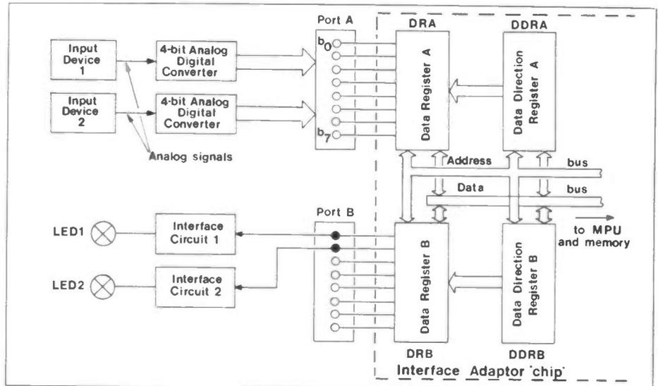
Figure 1. The Microcomputer as a Control Centre.
