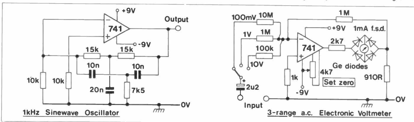
Figure 10. A test oscillator and electronic a.c. voltmeter
