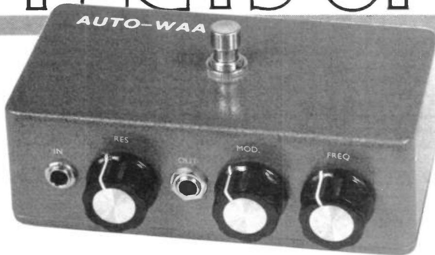
There are several ways of producing the well known and much used waa-waa effect, but in each case the basic effect is generated using some form of bandpass filter which is swept up and down over all or part of the audio band. This boosts a fairly narrow and continuously changing band of frequencies, and it is mainly the consequent variations in the relative strengths of harmonics in the processed signal that give the effect.
