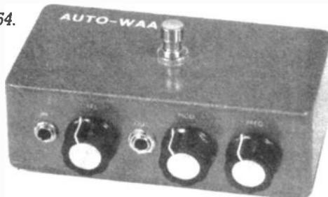
ially boosted as the filter sweeps through them, and with a high level input overloading with attendant distortion could result. There is also a danger of overloading the equipment fed from the output of the unit, and the best effect tends to be obtained with the filter sweeping over medium and high frequencies anyway.
