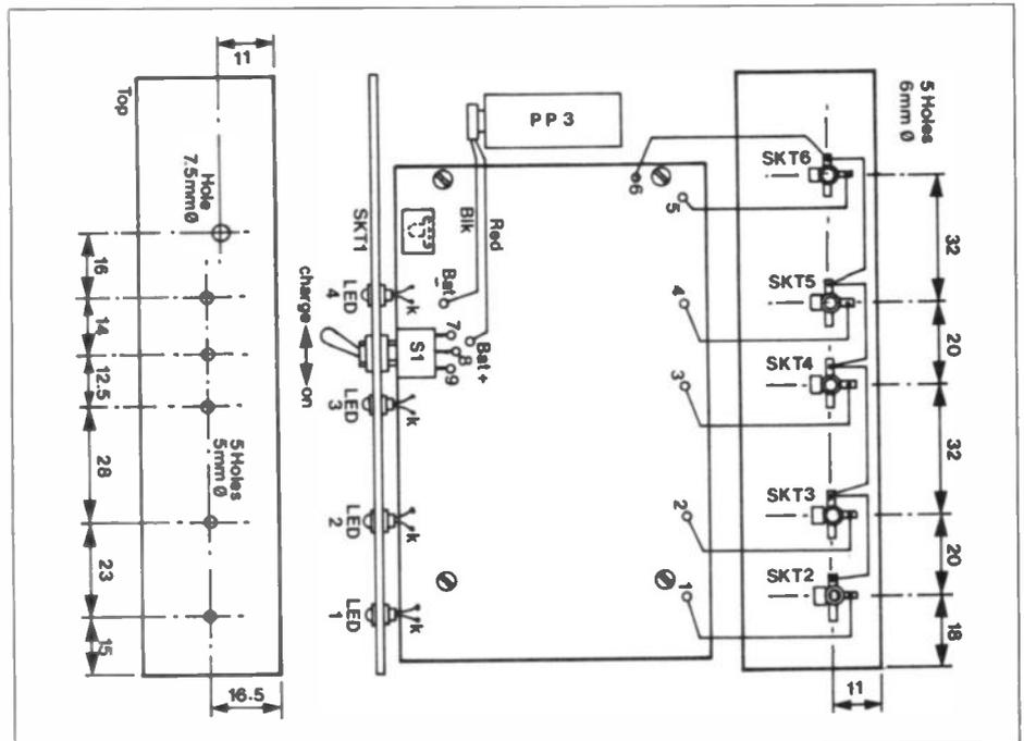
Figure 5. Box drilling
