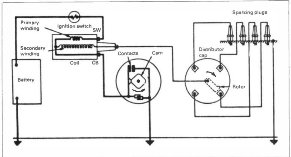
Figure 3.3. Sparking plugs firing circuit
