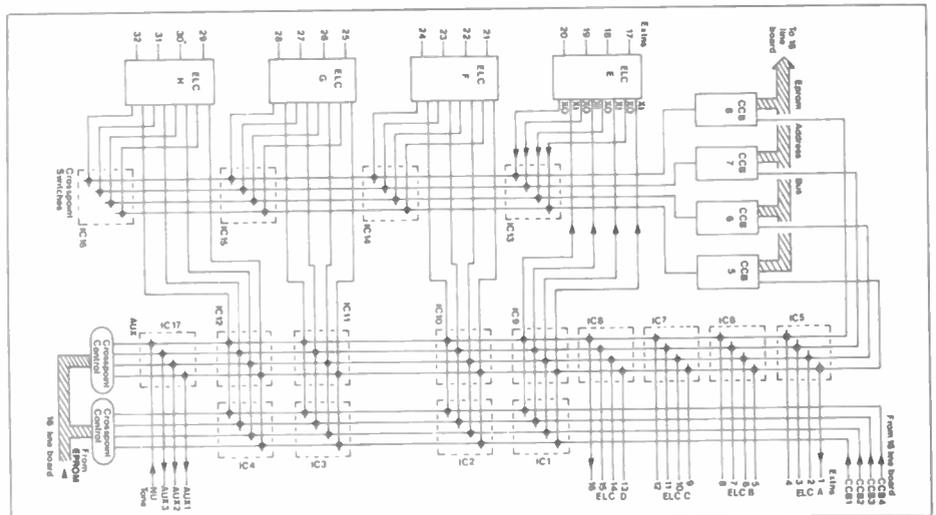
Figure 1. Block diagram of 32 line extension board
