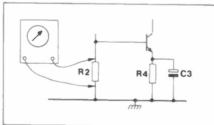
Figure 5. Measuring resistance 'in situ'.
