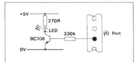
Figure 4. LED Driver Circuit.
