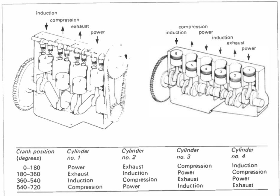
Figure 2.1. 4-cylinder and 6-cylinder engines
