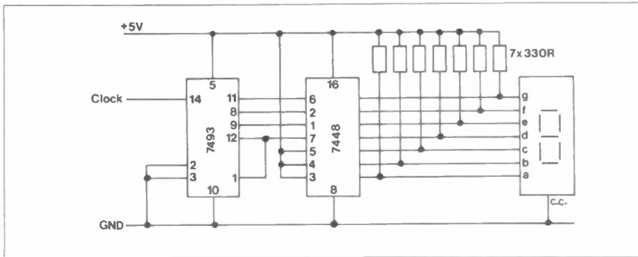
**Figure 8. TTL counter with 7-segment display output.**
