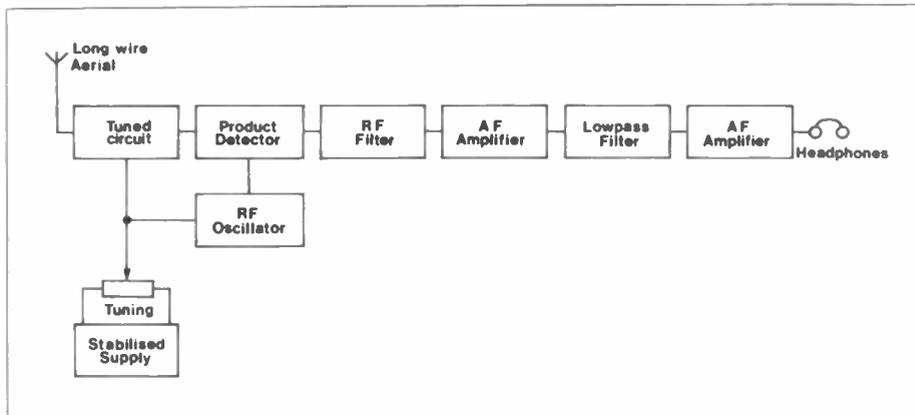
Figure 2. Block diagram of the Direct Conversion Receiver.
