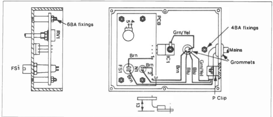
Figure 5. Assembly and wiring
