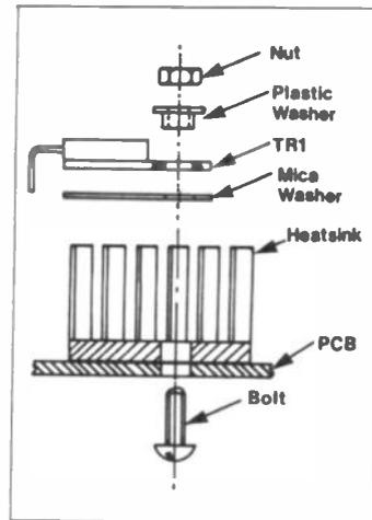
Figure 4. Mounting the transformer and heatsink
