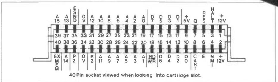
Figure 2. Cartridge slot pinouts.
