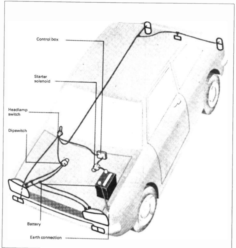
Figure 1.3. The lighting circuit
