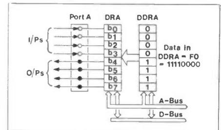
Figure 2. Configuring a Port for Input/Output Functions.
