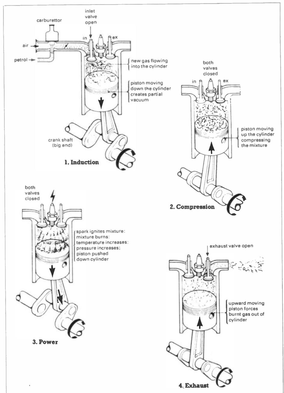
Figure 2.2. The four stages of combustion
