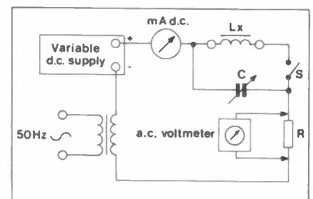
Figure 8. Turner's method for measuring large inductors.
