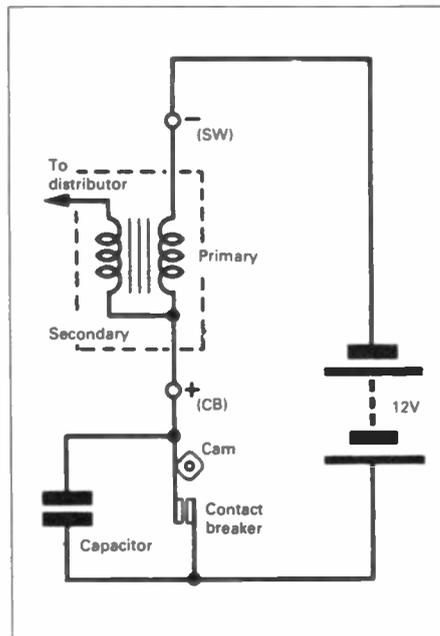
Figure 3.1. Basic high voltage generating circuit
