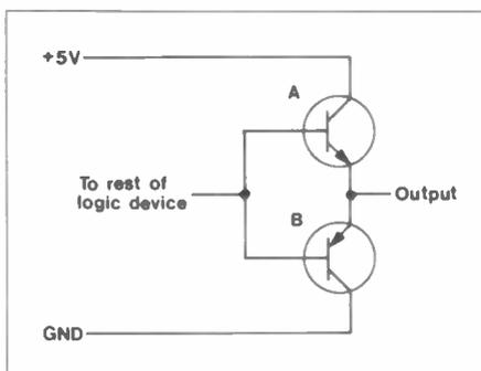
Figure 1. TTL output stage.
