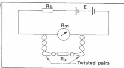
Figure 3. Arrangement to measure low values of resistance.
