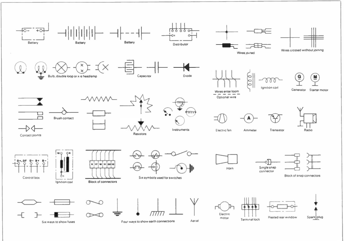
Figure 1.5. Common symbols used in car wiring diagrams
