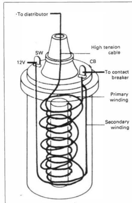
Figure 3.2. The ignition coil
