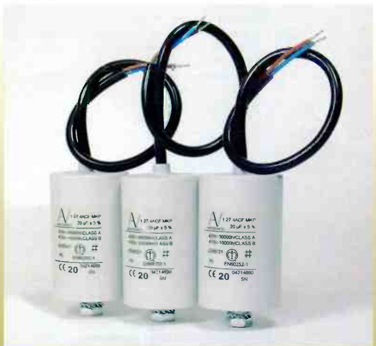
Three 'motor start' capacitors, of 20uF apiece. Connecting them across the secondary of the balancing transformer filters out mains borne noise and interference. This is another way to lessen noise input to the hi-fi system. Motor starts are high voltage polypropylene capacitors suitable for power work.
