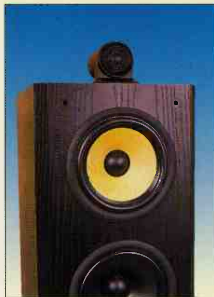
The light and fast yellow Kevlar cone lends a clear and open midrange to the 803s. Externally located tweeter was not in the same league.
