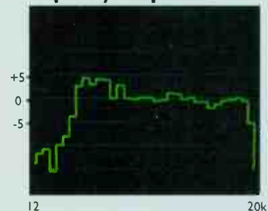
Bass starts to lift from 250Hz, otherwise the 803s have a flat response.
