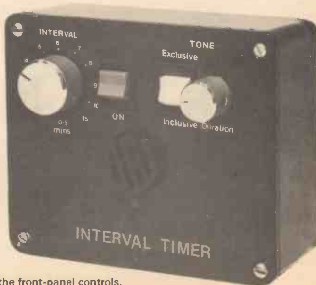
The Timer, showing the front-panel controls.
