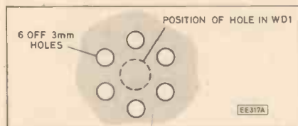
Fig. 5b. Suggested pattern of holes to be drilled in the case over the sound transducer.
