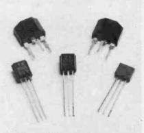
Fig. 2.8b. Transistors in plastic packages.
