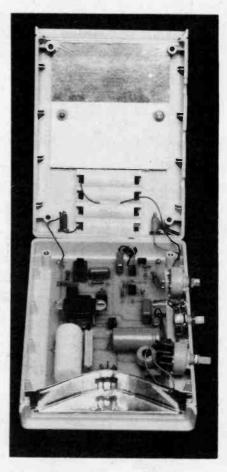
The completed prototype showing reflector in position and the controls seated in one section of the case. Note that SK2 and SK3 are mounted in the top half of the case as seen.
