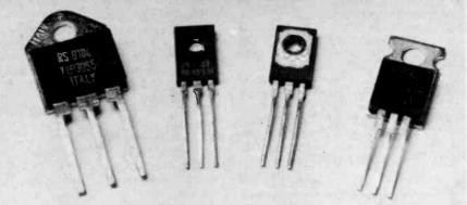
Fig. 2.9a. Plastic package power transistors. The two devices in the centre are in fact the two sides of the same package. The metal plate attached to the collector, designed to be bolted onto a heat-sink can be clearly seen.
