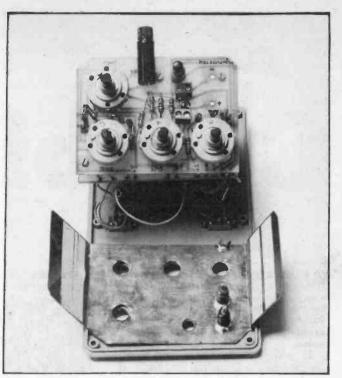
View of the rear of the front panel. The tinplate screen is shown mounted in position and the component side of board A is also shown. Note that the input sockets, SK1 and SK2 are still mounted in place on the front panel. When the circuit board is in position these solder directly into board A.
