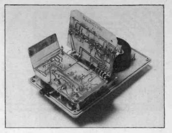
Board A is shown fixed in position mounted on the front panel, and board B is shown hinged back to reveal the wire links.
