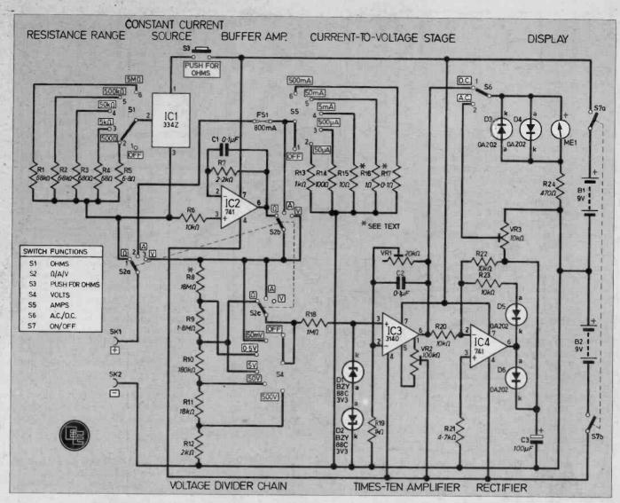
Fig. 1. Full circuit diagram for the Electronic Multimeter. Note that the meter ME1 is a 1mA f.s.d. type.
