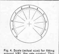
Fig. 4. Scale (actual size) for fitting around VR1, the rate control. This has been drawn to suit potentiometers with 270 degrees electrical rotation. happen switch off, discharge the capacitors as described above and investigate.
