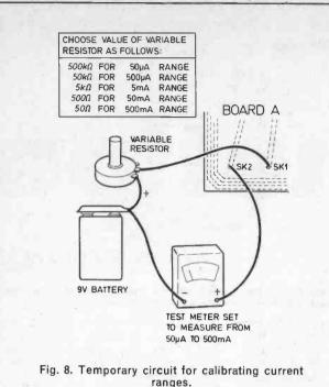
link sockets SK1 and SK2 together. The inputs to IC3 are now effectively grounded. Switch power to the multimeter by means of S7 and adjust trimmer VR2 until the meter reads zero. Switch off the multimeter, remove the short from the input sockets and return the range switches to off.
