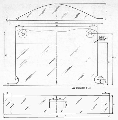
Fig. 5. Templates with dimensions marked for making a reflector to suit the specified case.
