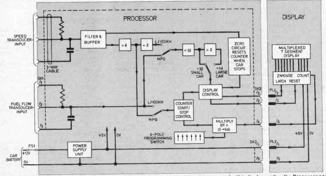
Fig. 1. Block diagram of the Fuel Stretcher. This shows the overall system and how it is arranged within the two units—the Processor and the Display.
