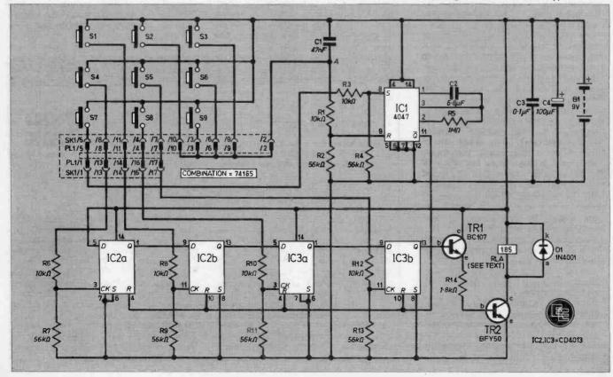
oscillator in the chip and setting the  $\overline{Q}$  output to zero. The internal bistable will count two oscillator pulses and then set the  $\overline{Q}$  output to logic level 1 (approximately equal to  $V_{\rm DD}$ ). The frequency of the oscillator is set by the value of capacitor C2 and resistor R4, and this is directly related to the period of the monostable.
