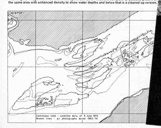
Map below shows the positions of sandbanks in the Bristol Channel plotted both by satellite and by conventional means. The disparity between the two can be clearly seen. The three photos to the right show part of the Wash and were produced using data from Landsat 1. The top photograph is an original image in the red end of the spectrum. Below that is a computer processed picture of
