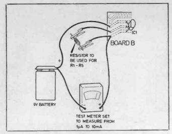
Fig. 5. Temporary circuit for selecting R1 to R5.
