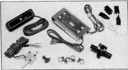
T HIS article describes a fuel consumption monitor for in-car use, designed to fit most vehicles with a carburetter fuel system and cable driven speedometer.
