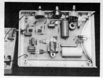
Plan view of the section of the case which holds the circuit board and emphasises the need for sleeving the tags on S2.
