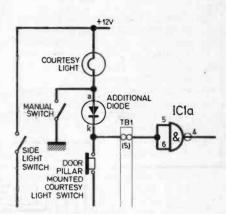
*Mr.* Burgess's suggestion for modifying the Lights Reminder and Ignition Locator for vehicles with a manual courtesy light switch. This has not been tested by us.
