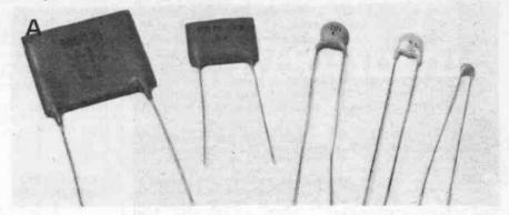
**B** A selection of different **plastic dielectric** capacitors. Top left is a **metallised polypropylene** film capacitor encapsulated in a flame retardent plastic case. This is a general purpose type of device, tolerance 20 per cent and voltage rating 400V d.c.
