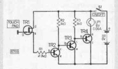
This circuit, which I thought of, uses an f.e.t. (field effect transistor) as a variable resistor. Depending on the amount of time that your finger is on the touch pad, this is the amount of time that the light, LP1, is on for. When the gate of TR1 is touched a few microamps flows into it and stops the flow of current from the drain to the source thus turning on the lamp. Transistors can be: TR1-2N3819; TR2, 3-BC107; and TR4-2N3702.
