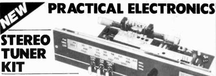
This easy to build 3 band stereo AM/FM tuner kit is designed in conjunction with Practical Electronics (July Issue). For ease of construction and alignment it incorporates three Mullard modules and an I.C. IF. System
