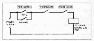
Fig. 3.2. Simplified circuit for an automatic gas central heating system.
