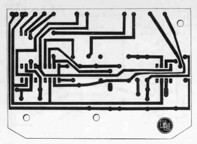
Fig. 2. (above) Foil pattern for board B full size. Foil pattern for board A is shown to the left on the facing page, also full size.
