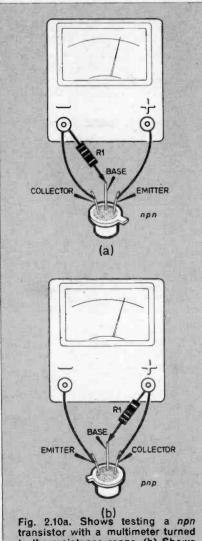
to the resistance range. (b) Shows similar testing of a *pnp* transistor.
