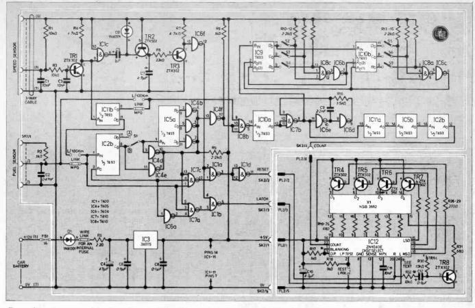
Fig. 2. Circuit diagram of the Fuel Stretcher. The Display Unit circuitry occupies the lower r.h. corner. Clarification of the connections to IC12 is given in Table 1.
