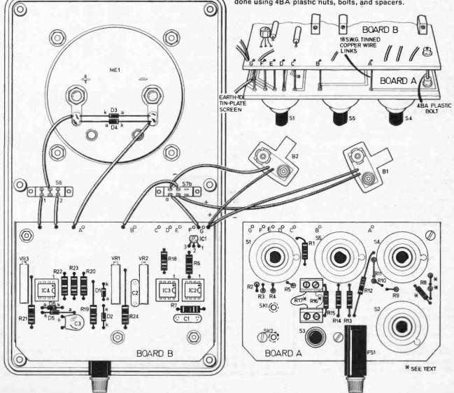
Fig. 3. (below) Component layout for board B and interwiring to certain off-board components,
