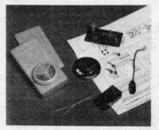
appropriate, loudspeaker(s), and in all but one kit a brightly coloured plastic case. All cases have an aperture for the loudspeaker which is "snapped" into position thereby eliminating the need for any form of hardware fixings, cutting or drilling thereby keeping construction as simple as possible. A neat solution!
