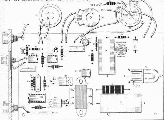
Fig. 3. The layout of the components on the topside of the circuit board and wiring details to the case mounted components. The tags on S2 are shown splayed for clarity.
