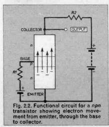
emitter. In many transistors about 99 per cent of the electrons from the emitter reach the collector, the other 1 per cent giving rise to the external current in the base circuit.
