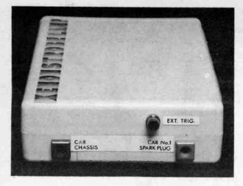
View of the rear face of the case showing the external trigger sockets clearly labelled.
