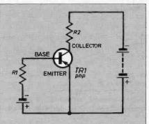
Fig. 2.4. Basic circuit for a pnp transistor
