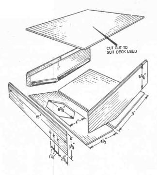
Fig. 6. Basic cabinet details of the prototype. This cabinet may be made to any design required. The back panel has not been shown but is rectangular with holes for SK1 and the mains lead.
