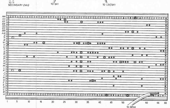
Fig. 4. Veroboard layout and wiring details. The board used is 0-1inch matrix.
