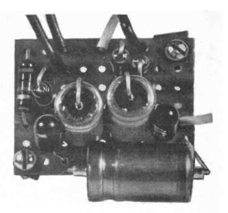
switching transient. The high back e.m.f. produced in the relay coil when TR2 is cut off (thus de-energising the relay) is prevented from damaging transistor TR2 by diode D1 providing a shunt path for the back e.m.f. Capacitor C4 suppresses any transients at the relay contacts caused by sparking and should be a high voltage type mounted close to the contacts.
