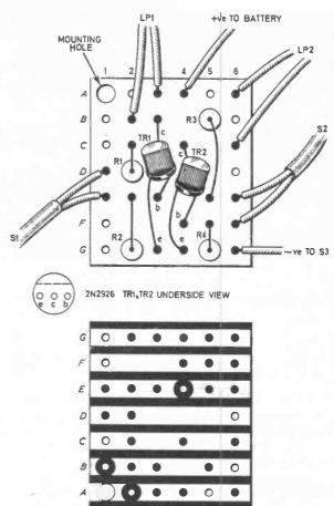
Fig. 2. Veroboard layout and wiring diagram showing both sides of the board and connecting wires
