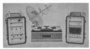
The latest ship-borne telemetery receiving equipment for receiving and processing of missile performance. The units shown are, from left to right, receiver, tape recorder and helical receiving antenna and the data monitoring cabinet (EMI)
