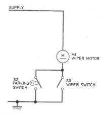
Fig. 5. Wiring diagram of a two wire field coil wiper motor with self parking facility.
