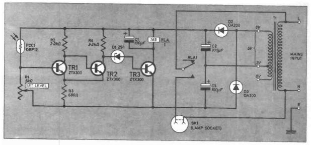
Fig. 1. Circuit diagram of the Home Sentinel. Relay is shown in position with the cell illuminated.
