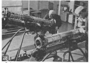
Submerged repeaters being finally assembled. In 1962 when this picture was taken, the transistor had made improvements to our communications systems by its employment in equipments such as these repeaters (S.T.C.)
