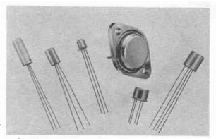
A selection of semiconductors, the development of which was to mean the demise of many valves. Small size, reliability and low voltage operation are the advantages of semiconductors (Mullard)
