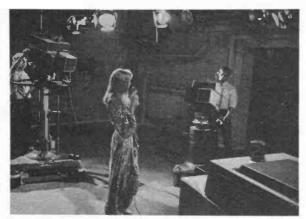
The first automatic colour television camera introduced in September 1970. Lengthy alignment and colour balancing routines necessary with previous cameras have been replaced by fully automatic corrections made by a miniature computer built into the camera channel (Marconi)
