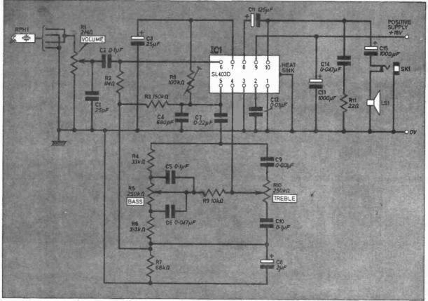
Fig. 1. Circuit diagram of the Record Player amplifier using a single integrated circuit.
