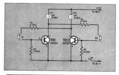
Fig. 1. Complete circuit diagram of the Snap Sequence Indicator.
