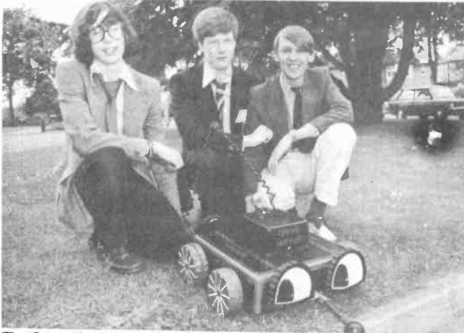
The Grass Hopper made its television debut in April on Tomorrow's World. Designed by Frank Carver, it's an admirably practical robot for armchair gardeners — it cuts grass. The design team, from Farnborough 6th form college have since produced a Mk 2 CMOS version.
