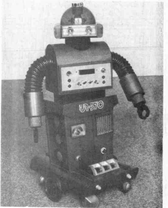
UR370 started life as a two channel Futaba radio and a pound of splintered balsa wood. Both the UR 700 and its brother, the UR 370 are designed by Joe Gillespie.
