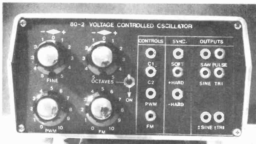
Above and below: the VCO and PSU modules as they appear in their free standing cases. Note the vernier drive on the PSU. This is for calibration of oscillators etc. This case will be standard throughout the series.
