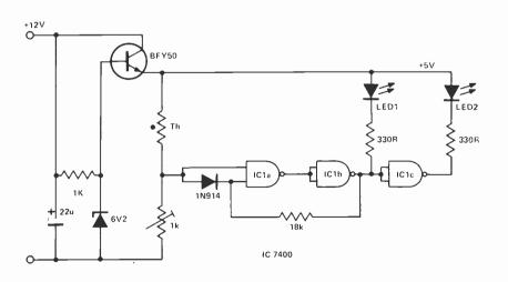
temperature falls, all gates change state, LED2 goes off and LED1 (red) comes on The temperature at which the changeover takes place is set by the 1k preset.
