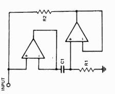
be added except that the Q of the circuits must be changed to narrow the band. At the moment the impedance of the capacitor and inductor (gyrator) is about 3000 ohms at the centre frequency and this should be increased to about 8000 ohms for the third octave unit. The capacitors and inductors can be calculated by  $C = \frac{1}{2\pi f X_c} \quad L = \frac{XL}{2\pi f}$ where X<sub>C</sub> = X<sub>1</sub> = 80000.
