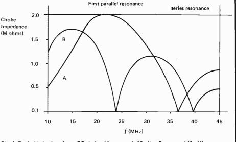
Fig. 4. Typical behavior of two RF chokes (A = around 10  $\mu$ H, B = around 40  $\mu$ H) over a range of frequencies.
