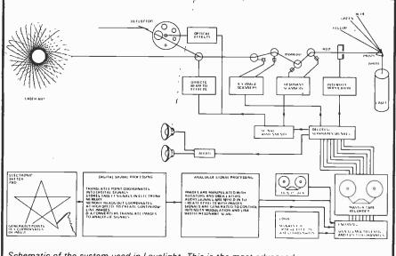
Schematic of the system used in Lovelight. This is the most advanced system in use at the moment. The scanner network is duplicated for the three other colours shown.
