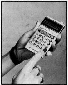
Made to slip into a pocket or handbag, this new CBM LCD calculator is only 1/4inches thick. Called the LC5K1 and obviously aimed at the female half of the human race, the case is a nice 'posh' brushed beige metal. Based on a 3 volt CMOS chip, its power consumption is very low, giving the battery an anticipated life of 5,000 hours. (This means that if you left it on accidentally, it would still be working seven months later - handy if you're prone to a long unexpected illness!).
