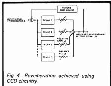
Differing path lengths are arranged using different delays. Specific attenuation in a path represents acoustic absorption loss which, by its adjustment, allows for the overall control of delayed reverberation time.
