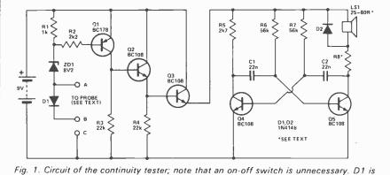
used when the battery is brand-new and giving over the nominal 9V Q1, Q2 and Q3 act as the switch for supplying power to the multivibrator.
