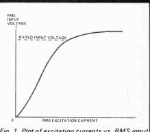
Fig. 1. Plot of excitation currents vs. RMS input voltage for typical transformer. The transformer should not be operated for long periods above the knee of this curve.
