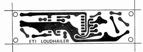
Fig. 3 PCB pattern (105mm x 30mm)
