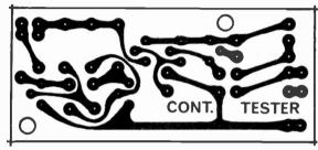
Fig. 2. The pcb pattern shown full size (73mm x 33mm).
