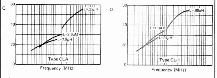
Fig. 7. Typical Q values versus frequency for several values of two different sizes of moulded RF chokes (From IRH). CLA = 6.4 mm dia. x 78 mm long. CL1 = 6.4 mm dia. x 27 mm long.
