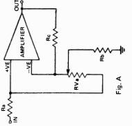
It must be emphasized that this equivalent circuit represents the condition with one filter only, at its resonant frequency. Additionally letters have been used to designate resistors to avoid confusion with components in the actual
