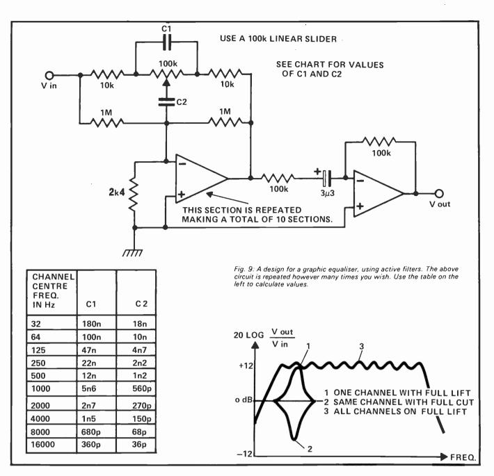
shows a common tone control with just bass and treble functions. Again cut and lift ranges are 20dBs. If a more flexible control of the spectrum is needed then a ten band graphic equaliser (Fig. 9) could come in handy.
