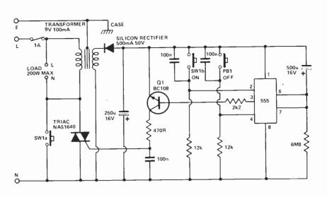
it must be rated accordingly. SW1b is used to trigger the 555 and start the timing period.'Q1 will then be turned on, providing gate current to turn on the triac. When SW1 is released the supply and the load is maintained until the end of the timing period. PB1 is provided so
