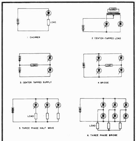
Fig. 10. Various inverter configurations using SCR switches. Triggering methods have been omitted for clarity.
