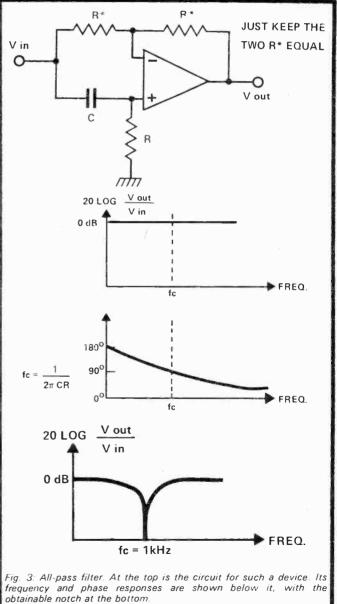
If we then mix the phase delayed signal with the original, a notch response is obtained. This is because at fc the two signals have the same magnitude, but the opposite phase and so they cancel each other out.
