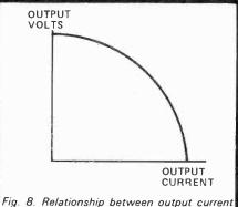
and output volts of high reactance transformer with resistive load.
