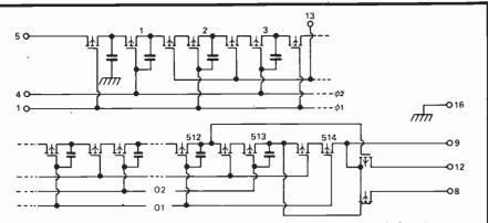
Fig 6. Internal circuitry of the Mullard TDA 1022 Bucket Brigade chip. The pin functions are as follows: Clock input (V<sub>CL2</sub>), 2. NC. 3. NC. 4. Clock input (V<sub>CL2</sub>), 5. Signal input. 6. NC. 7. NC. 8. Output 513. 9. V<sub>DD</sub>. 10. NC. 11. NC. 12. Output 512. 13. Tetrode gate. 14. NC. 15. NC. 16. Ground.
