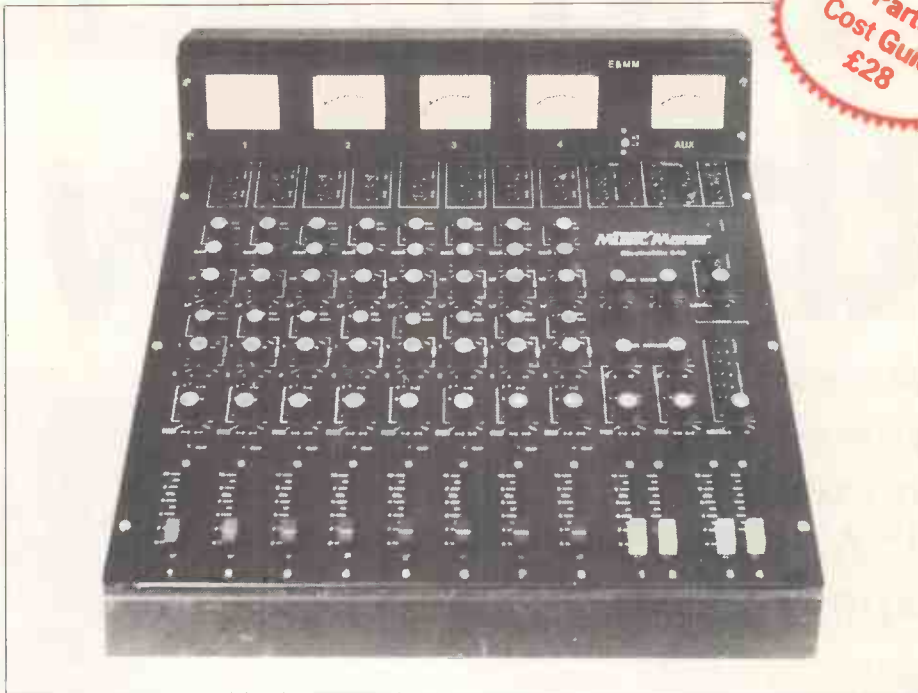
Meter bridge fitted with The ElectroMix 842.
