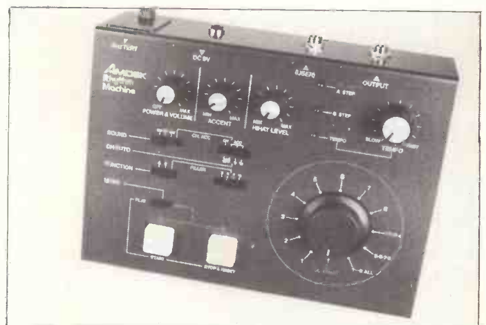
The completed Rhythm unit with knobs and switch tops added (Steps 19-22).
