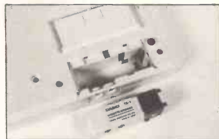
TA-1 Interface ready for installation in MT-65.
