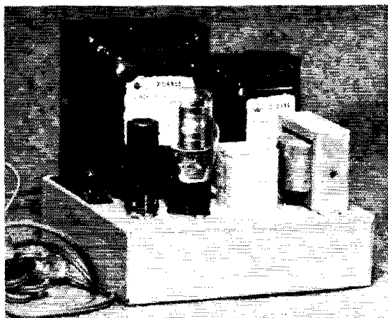
The power supply is assembled on a 7 \times 7 \times 2 -inch chassis. The bias transformer is between the OA3 voltage regulator and the low-voltage filter choke. Diodes, filter capacitors, and resistors are inside the chassis.
