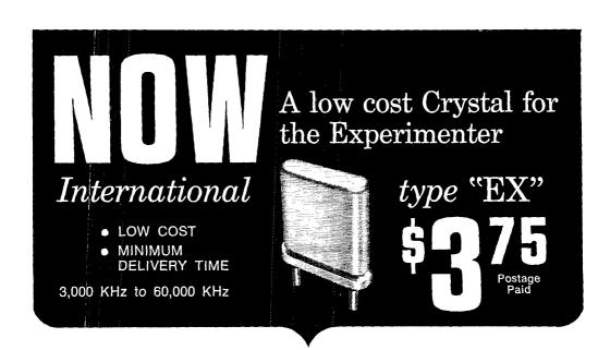
**SPECIFICATIONS:** International Type "EX" Crystal is available from 3,000 KHz to 60,000 KHz. The "EX" Crystal is supplied only in the HC-6/U holder. Calibration is  $\pm$  .02% when operated in International OX circuit or equivalent.
