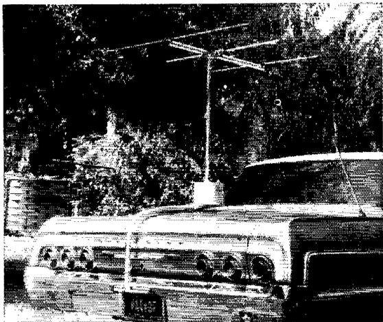
This novel 2-meter mobile antenna belongs to WA4WBF at Winter Haven, Florida. The Yagi is rotatable from driver's seat by means of an electric automobile window motor. The whole assembly can be put on, or taken off, the car in one minute.
