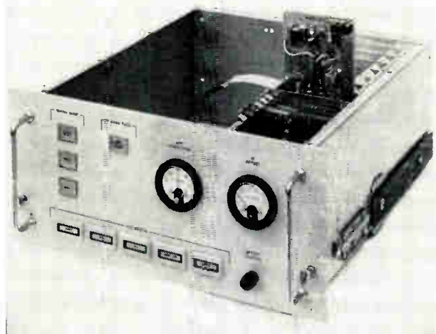
Fig. 1: A partially assembled chassis with mixed frequency modules is typical of the module design.
