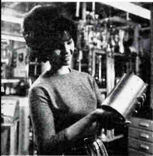
This 19-lb. superconducting magnet can duplicate the performance of a 600-lb. conventional Alnico V permanent magnet. It was designed and produced by The Arnold Engineering Co., Marengo, Ill., a subsidiary of Allegheny Ludlum Steel Corp.
