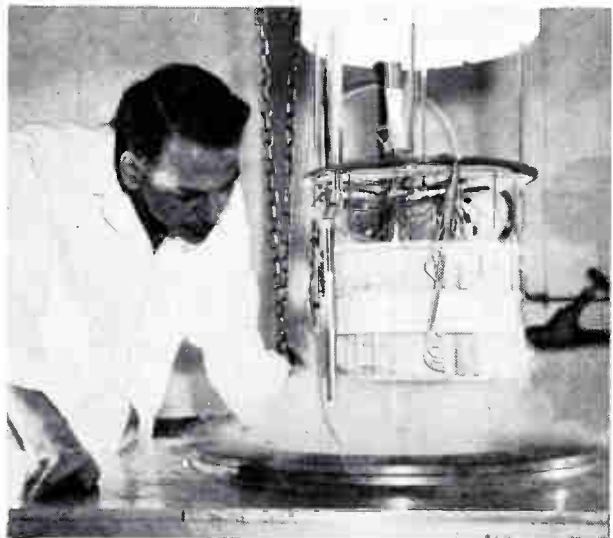
Avco SC600 superconducting magnet is lifted from its -450°F liquid helium bath after a test run. Coil is wound with niobium-zirconium and multiple insulation. Coil ID is six inches.
