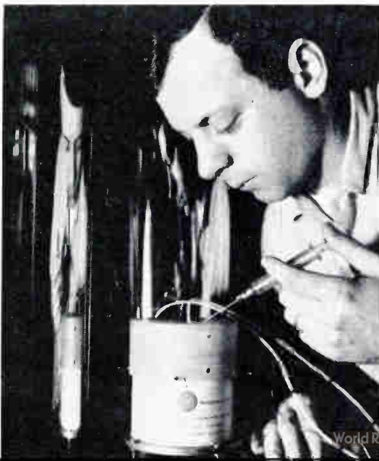
Engineer (below) works on a Westinghouse superconducting magnet. This magnet has a field rating of 50,000 gauss. Its rated current is 12.70 amps.
