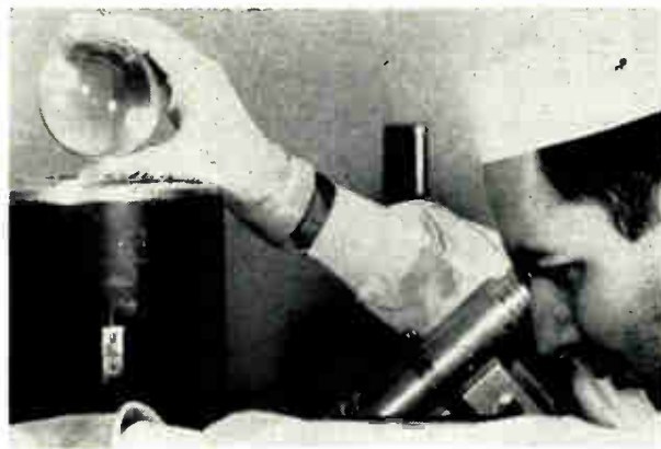
Fig 1: One optic device is checking another. Roundness of ball can be checked within 2 millionths of an inch.
