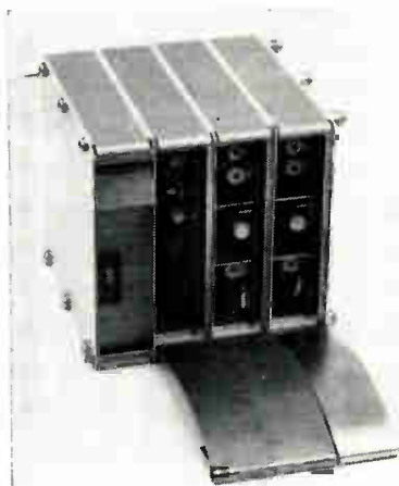
Fig. 2: A clear view of three i-f modules in place with the spring covers open.
