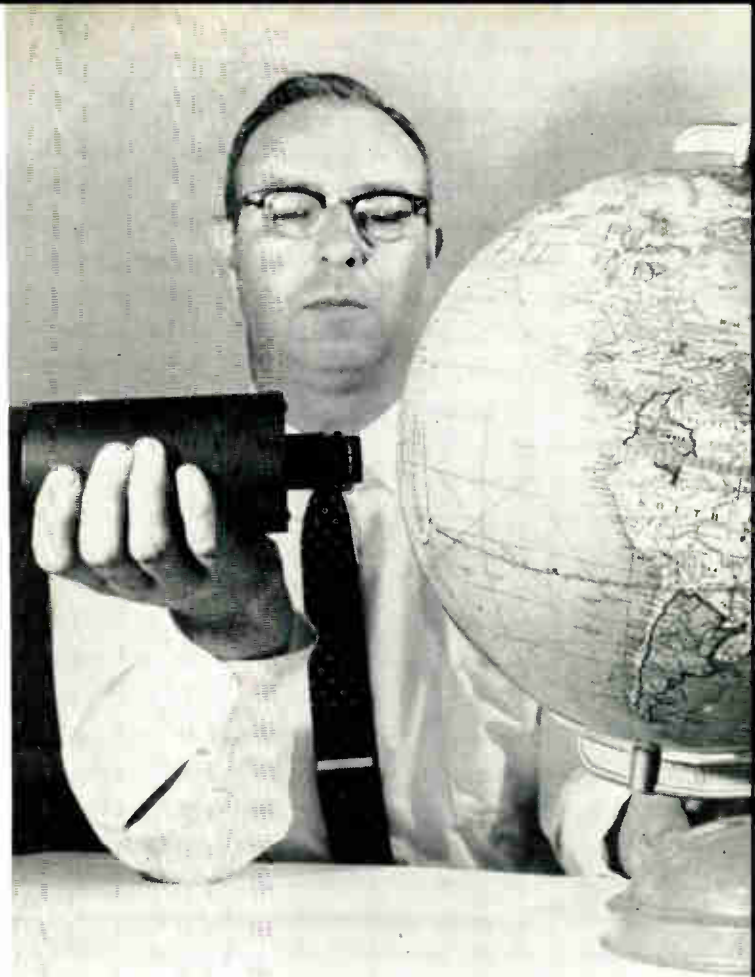
Fig. 2: The "attitude sensor" is a small electronic mirroring device that can correctly position huge orbiting satellites on less power than that needed for a miniature flashlight bulb.
