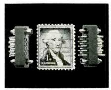
This connector line features: Diallyl Phthalate molding; 1-piece 3-48 thread screwlock; bow washers to eliminate axial float; square shoulder in molding for fixed screwlock; strengthened "C" clip groove; and controlled float in socket contact. The mounting pad surrounds the entire guide hole. Both male and female contacts are of phosphor bronze. The MM22 Series meets applicable Mil specs. Lionel Electronic Laboratories, Inc., 1226 Flushing Ave., Brooklyn 37, N. Y.
