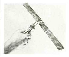
Line of permanent cable ties called STA-STRAP combines self-locking Nylon cable ties and clamps with a tensioning tool that automatically cuts off excess strap at a pre-set tension. The STA-STRAP is installed by threading the tip through the eye. The Panduit Tool is squeezed to accomplish final controlled tie tension and flush cut-off by excess strap. No twisting, pushing or pulling is required. Panduit Corp., Dept. ES-2, 17301 Ridgeland Ave., Tinley Park, Ill
