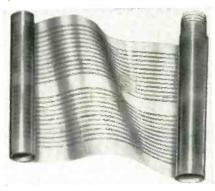
The conductors are encapsulated in Mylar. The material, a new variation of Methode's Plyo-Duct, is available in continuous lengths and contains up to 24 pairs or 48 conductors of 0.002 in. round copper wire. This wire, in a film 0.004 in. thick, has spacing tolerances of 0.002 in. Plyo-Duct has high dielectric strength under severe environmental conditions, with very good flex-life and min. weight characteristics. Methode Electronics, Inc., 7447 W. Wilson Ave., Chicago 31, Ill.
