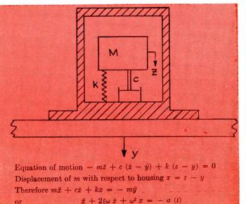
tained. In either case, almost all the pickups are single-degree-of-freedom systems (Fig. 1). Their performance can be determined from the differential equation:
