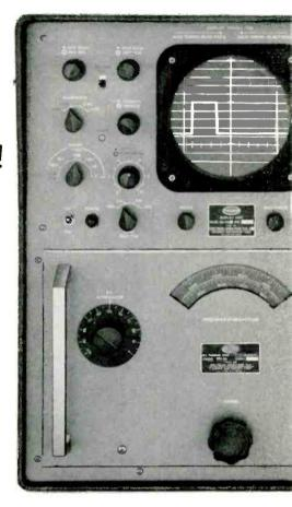
YOU SEE PULSED SIGNALS IN THE TIME DOMAIN IN THIS SYNCHROSCOPE MODEL TSA-S
