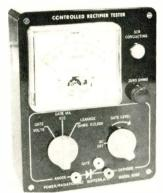
This portable unit determines the gate voltage required to fire the SCR (up to 5v); the gate current required to fire the SCR (up to 50ma); and the anode-cathode or anode-gate leakage (up to 8megs). It comes complete with color coded test leads, and operating instructions. The unit operates from 115v, 60CPS. Size is  $5^{14}$  x 3 in. Weight is approx.  $2^{1/2}$  lbs. Power/Radiation, Inc., Box 616, Suffern, N. Y.
