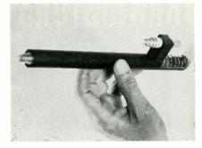
The L-3711 is a metal-ceramic TWT featuring 36db min. small signal gain and high linear saturation characteristics. It is conductioncooled, measures  $12\frac{1}{2}$  in. long and 7/8 in. in dia. and weighs 21 oz. It operates with temp. compensated periodic focusing and also features high linear power. Helix design and fabrication techniques have raised the saturation gain to within 3db of small signal gain. Litton Industries, Electron Tube Div., San Carlos, Calif.
