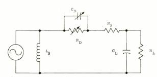
Fig. 2: Equivalent for relaxation oscillation circuit of Fig. 1.
