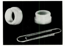
It provides mechanical mounting of the transistor without the need of a socket on metal chassis. The Sealectro B-1470 (Teflon) Transistor Bushing is pressed into a prepared hole 0.4 in. in dia. The Bushing is hollow, with a lead hole of 0.330 in. in dia. for connection of transistor leads. The receptacle for the transistor body is 0.300 in. in dia., and is chamfered for easy inserting. Height above chassis is 0.120 in. Sealectro Corp., 139 Hoyt St., Mamaroneck, N. Y.
