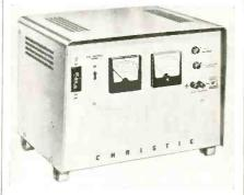
Six models offer a continuous voltage adjustment range of 1 to 145vdc and up to 50a. Standard ac supply source required is 115v, 1  $\theta$  60CPS. Unit available for 230v, 1  $\theta$ , for 50, 60, or 400CPS and even for all 3 freqs. combined. All models are regulated against line and load variations and have an adjustable automatic battery charging and other constant voltage or constant current uses. Christie Electric Corp., 3410 W. 67th St., Los Angeles 43, Calif.
