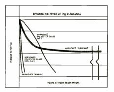
At 12% elongation "Fibremat" retains a substantially greater percentage of its original electric strength than either woven cambric or polyester-glass materials. This basic ability to retain electric strength means less insulation thickness is needed with "Fibremat" to attain the same electrical performance achieved with heavier layers of old style materials. Less insulation and less labor is required to finish a component. Insulation costs are reduced!
