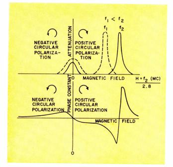
Fig. 3: Some typical phase and attenuation characteristics plotted as a function of the direct current field strength which is applied. Weiss<sup>22</sup> has also suggested that the proper modulation of the dc field might lead to early appearance of subsidiary resonance. This would make very low level limiters possible.
