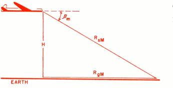
Fig. 1: The Idealized cosecant-squared pattern lies uniformly along the surface of the (flat) earth.
