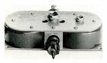
Millimeter wave tubes have found uses as microwave spectroscopy signal sources, maser pumps, power sources for CW or pulsed doppler radars, harmonic generators, local oscillators, in gas plasma experiments, commercial moisture detectors, inter-satellite communication systems, ballistic missile to ground telemetry systems, as well as signal sources for antenna design experiments.
