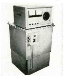
Input requires 105 to 125vac, 60CPS. The instrument and control center, mounted on the high voltage assembly tank, may be used at a remote point. The instrument and control center contains complete metering, overload protection, switches and indicators, as well as the output control. The high voltage assembly tank with casters measures 24 x 24 x 40 in. The control center measures 21 9/16 x 14 7/8 x 13 in. Plastic Capacitors, Inc., 2630 N. Clybourn Ave., Chicago, Ill. Circle 335 on Inquiry CARD
