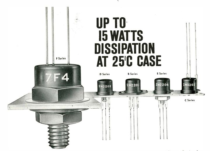
For high power dissipation in a small area, these new General Electric silicon mesa power transistors have no equal for aircraft servo or missile applications. Four combinations of electrical characteristics are available in five different package designs to meet your particular circuit requirements. And all feature (except 7F series) 15 watts power dissipation at 25°C case temperature.
