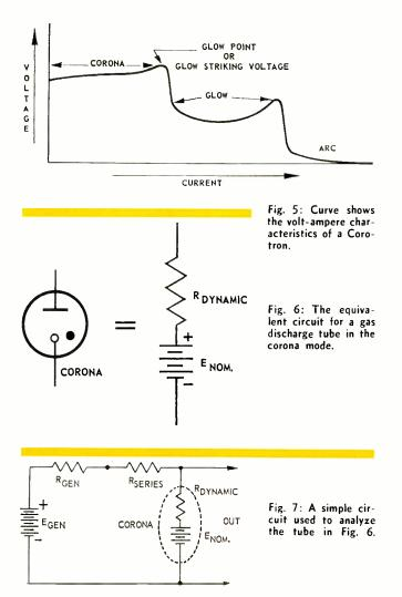
regardless of initial energy, the tube is acting as a Geiger tube. The current is now proportional to the number of events-per-unit of time rather than total energy. The current depends upon the external energy —it would be zero without that energy.
