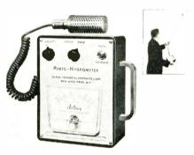
The Jelrus PORTO - HYGROM-ETER is a portable battery-operated humidity indicator. By pushing a button, instantaneous and direct relative humidity (R.H.) is read from 30% to 100% with a single electronic sensor and dial. Extension rods of varying length permit direct reading of R-H in hard-to-get-at spots, within  $\pm 5\%$ . The unit is unaffected by barometer changes. It will with-stand rough use. Jelrus Technical Products Corp., 2020 Jericho Tpke., New Hyde Park, N. Y.
