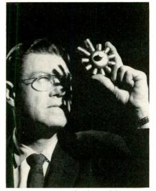
Raytheon Co. space Amplitron delivers more power per pound. Radical design permits use of single small magnet for the tube which delivers 25w, yet weighs only 16 oz. Efficiency of 60%, combined with light weight and compact design make the new Amplitron ideal for space communications systems.
