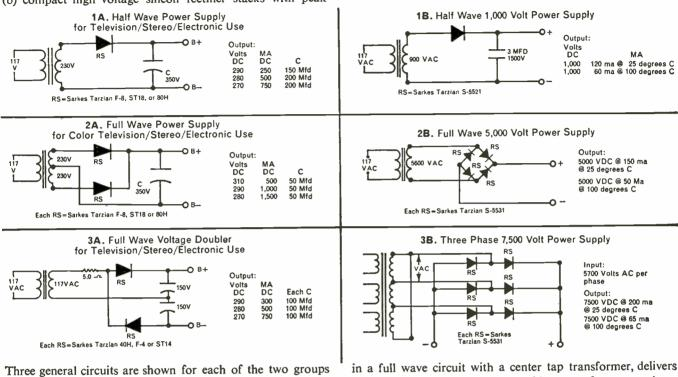
mentioned above to suggest some of the possibilities. For example: 1-A, a simple half-wave circuit operating off a 230 volt line or with a 1 to 2 step-up transformer, delivers between 270 and 290 volts with a capacitive input; 2-A, with two rectifiers
