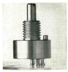
The JP/2 is a panel mount potentiometer, smaller in overall volume than standard  $\frac{1}{2}$  in. miniature pots and considerably lower in cost. It is designed to meet standard military environmental specs. The JP/2 can be interchanged with most  $\frac{1}{2}$  in. pots. It is available in a resistance range from 10 $\Omega$  to 20K $\Omega$ . Waters Manufacturing, Inc., Wayland, Mass. Circle 355 on Inquiry Card
