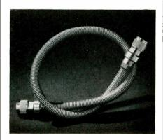
AMPHENOL ultra-high temperature flexible rf cable is capable of continuous operation at 1000°F with short excursions to higher temperatures. Application engineered for aircraft and missile temperature environments, the cable is a completely sealed rf transmission system consisting of inner and outer conductors separated by a dielectric of modified semi-solid silica.
