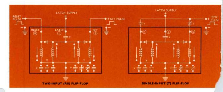
The "X" and "Y" coils of the two-input (RS) flip-flop are double wound and are diode coupled in opposition so as to produce zero flux when both windings are energized. One winding of each coil is connected to one Clareed switch of the "X" coil for latching.
