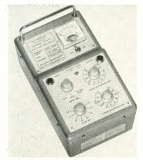
It is a fully transistorized, self-contained, battery-operated amplifier. Noise, with 50meg input, open or shorted, is less than  $3\mu v$  with a bandpass of 10KC. Unit has other input impedances of 10 and  $100k\Omega$  for use with lower source resistances. Amplifier has 80db gain with 10db steps. Max. output is lv RMS on any gain setting. Freq. response is 2CPS to 180KC. Millivac Instruments, Inc., P.O. Box 997, 1100 Altamont Ave., Schenectady, N. Y.
