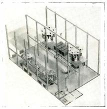
Artist's sketch shows arrangement of space chambers in the new space environmental lab being built by Hughes Aircraft Co. in El Segundo, Calif. Four of the chambers will be installed initially, with room for two more. The largest, with a test volume of 14 ft. in diameter by 15 ft. high, can accommodate a full-size Surveyor spacecraft for study under a space environment.
