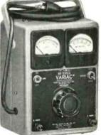
W5MT3W VOLTMETER/WATTMETER COMBINATION
