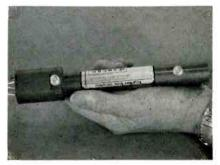
Of almost identical and rugged design, both tubes are of metal-ceramic construction, are PPM focused and feature a  $7\frac{3}{4} \times 1\frac{3}{8}$  in. O.D. package complete with heat sink. The 314H has a power output of 2-3w at 25-27% efficiency and 27-33db gain over 1.5-3.0GC. The 349H has a power output of 10-15w at 25-30% efficiency and 25-30 db gain over 2.0-4.0GC. Hughes Aircraft Co., Microwave Tube Div., 11105 S. La Cienega Blvd., Los Angeles 45, Calif.
