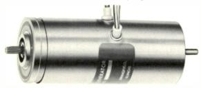
**NEW FEATURE ADDED TO SIZE 10 and 11 MOTOR GENERATORS** Sangamo's standard size 10 (.938" dia.) and size 11 (1.062" dia.) servo motor generators are now available with a rear shaft extension to permit mechanical coupling and/or speed checks after the unit is installed. Positive alignment is assured by the use of three ball bearings in each unit.
