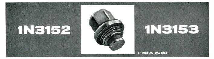
These 250 milliwatt diffused silicon diodes come in vacuum-tight hexagonal cases which are threaded for screw mounting and are particularly suited for strip line application.
