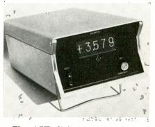
The ASX digital voltmeter measures 5¼ x 8½ x 14 3/16 in. This size allows for internal mounting of such optional equipment as ac/dc converter, battery pack for isolated dc operation, ratiometer, ohmmeter, automatic range and polarity, and printer drive. The voltmeter is in 3 basic models. These consist of completely solid state, reed relay and stepper switch units. Accuracy of each instrument is 0.01% of full scale ±1 digit. American Space Exploration Inc., 3910 S. Kalamath, Englewood, Colo.
