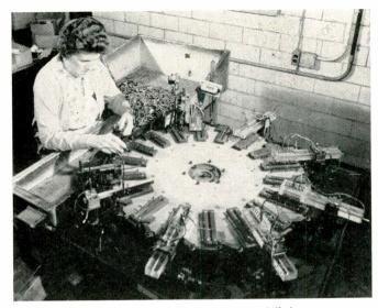
On this special automated equipment, a semi-skilled operator tests more than 2,000 custom-made, packaged assembly circuits per hour.
