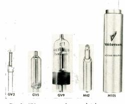
Fig. 3: HV power supply control tubes.
