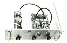
Stoddart R-F Step Attenuators use the "Pull-Turn-Push" turrent control. They are for use with standard  $50\Omega$ coaxial cable circuits, and are available in either 2 or 3 turret models. These attenuators have high accuracy from dc to 3GC with a very low phase shift characteristic at i-f freqs. up to 160MC. VSWR is less than 1.5 overall. Stoddart Aircraft Radio Co., Inc., 6644 Santa Monica Blvd., Hollywood 38, Calif.
