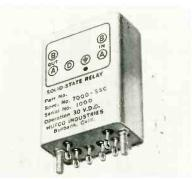
A SPST relay, with a contact rating of 1a, it operates on an input voltage of 10 to 30vdc. Contact voltage freq. range: from 300CPS to 30KC. Pickup time is 1msec. for relay latching, and dropout time is 2msec. after removal of contact voltage. Unit withstands temperature from  $-55^{\circ}$ C to  $+100^{\circ}$ C, with special models to  $+125^{\circ}$ C. Weight is less than 2 oz. Multipole ac or dc types are also available. Hufco Industries, 2815 W. Olive Ave., Burbank, Calif.
