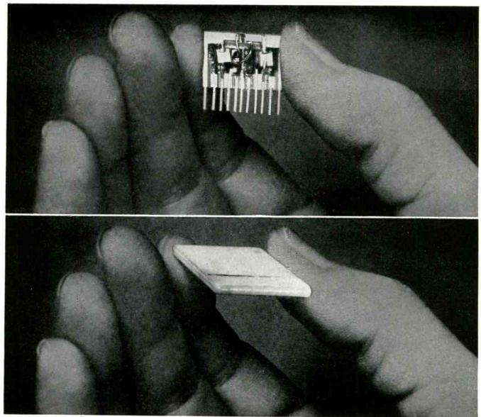
Micro-electronic welds to nickel-plated peramic substrate (top) and two edge-welded aluminum oxide ceramic wafers (bottom) show versatility of Hamilton-Zeiss Welders.
