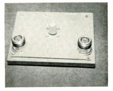
These switches are for receiver protection. Designed for uses from 100 to 2000MC, these reactive coaxial transmission line units handle more than 10kw peak power in the isolating state. Operating temperature is  $-55^{\circ}$  to  $+65^{\circ}$ C. A typical unit, Model SL5, operates over the band 1250-1350MC and has a minimum of 25db isolation in the forward bias state and a maximum of 0.5db loss in the back bias state. Hyletronics Corp., 185 Cambridge St., Burlington, Mass.
