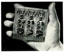
These plug-in modules permit low cost data transmission via cable over distances to 1000 ft. The modules operate at 200KC and are complete, except for a power supply, on 4 x 4 in. etched circuit cards. Model DT 100, the transmitter, can transmit, simultaneously, on 3 channels. Model DR 100, the receiver, also has 3 circuits, transformer coupled at the input, for ground and power isolation between transmitter and receiver. Packard Bell Computer Corp., 1905 Armacost Ave., Los Angeles 25, Calif.
