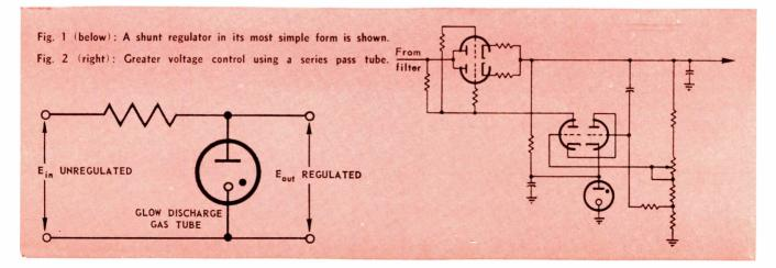
Voltage regulation and stability are the prime considerations in the design of power supplies. In the design of high voltage power supplies these problems have been considered particularly formidable. Only, however, because the components suitable for this work, as well as the design techniques, have not been fully understood.
