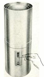
This line of diversionary Netic and Co-Netic magnetic shields use 2, 3 or 4 concentric cylindrical shields, one inside the other. The shield illustrated is 36 in. high and 15 in. O.D. It consists of 3 inner shields of high permeability Co-Netic alloy and 1 outer shield of heavy gauge Netic alloy. For viewing the sample under cryogenic test, a multi-section viewing port is provided. Magnetic Shield Div., Perfection Mica Co., 1322 No. Elston Ave., Chicago 22, Ill.
