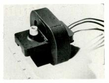
Designated the ZM-6050, it covers the 2.2 to 3.85GC freq. range and has a CW power output of 2w. Used as a local oscillator or a signal generator for rapid sweep applications such as radar and electronic countermeas-ures. The tube's low noise figure is the integrated noise in a band from 100KC to 100MC on both sides of the carrier freq. It weighs 3.5 lbs. and can be installed in any position. General Electric Co., Power Tube Dept., Schenectady, N. Y.
