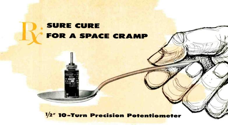
Spectrol's new miniature 10-turn precision potentiometer is a  $\frac{1}{2}$ " diameter pot with terminals located on the rear housing lid, eliminating side projections. Available in either bushing, servo or screw mount, the Model 160 is ideally suited for applications where excellent resolution is needed in a small package. Compatibility with a size 5 servo motor makes servo control a natural for the Model 160.
