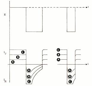
Fig. 7: The recovery characteristics of a junction diode to a long pulse and a short pulse for various values of forward current. With the large forward currents, the recovery time becomes greater.
