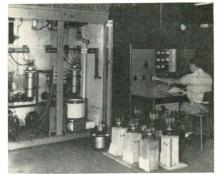
A linear amplifier test set for testing low mu factor, high perveance, high-power audio, and ultrasonic power tubes is shown in operation at the Westinghouse electronic tube division, Elmira, N. Y. Operator at the equipment console is matching two water-cooled tubes.
