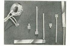
The TERMI-FOIL terminal is designed to reduce costs and improve performance of electrical equipment using aluminum foil and strips. It eliminates surface preparation. When the terminal is pressed into the foil by flat surface dies, tab projections pierce the foil, then fold over, securely riveting the foil to the surface of the terminal. The terminal will cover aluminum sheeting from 0.002 to 0.035 in. and can be spliced to 12-10 size wire. AMP INC., Harrisburg, Pa.
