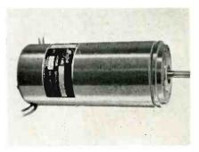
The V896-26B high performance servo motor generator is temperature stabilized by magnetic amplifier control to assure consistent accuracy despite temperature variations. Typical mechanical data includes: 4500RPM minimum no load speed; 2.35 in. oz. minimum stall torque; 35gm cm<sup>2</sup> rotor moment of inertia; and 4730 radians/sec. theoretical acceleration. The V896-26B weighs 27 ounces. Kearfott Div. General Precision, 1150 McBride Ave., Little Falls, N. J.
