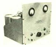
model E-4s regulated power supply may be mounted in a standard relay rack or installed in a cabinet for bench applications. Ripple is less than .05 volts peak to peak with an input between 105 and 125 volts, 60 cycle, 750 watts. There is less than a .15% varia-tion in output from no load to full load.— **Chatham Electronics Corp., 455 Washington** St. Newark N. 4. Newark, N. J.
