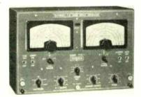
graph for visual alignment of television or FM radios. It provides a complete range of frequencies for the alignment of RF, oscilla-tor, IF and trap circuits. Sweep frequencies are from 2 to 216 MC in 3 convenient ranges, all on fundamentals. Sweep width is adjus-able from 100 KC to 12 MC bandwidth, ample width for the alignment of badly detuned erreuts.-Jackson Electrical Instrument Co., 18 South Patterson Blvd., Dayton 1, Ohio.
