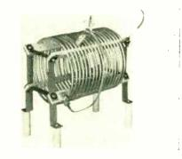
phasing and tuning equipment. RF heating equipment and heavy current filter circuits. These inductors are variable by means of tapping clips which may be either of the shorting or non-shorting type. Nominal inductances of 19, 38, and 65 microbenries are available in 10 anipere inductors: 20 anipere inductors are rated at 36, 53, and 76 microhenries, while the 30 ampere series are rated at 35, 49 and 71 microhenries.—Andrew Corp., 363 East 73th St., Chicago 19, 111.
