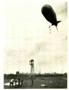
A helium-filled balloon carrying a pulse transmitter and antenna is raised by RCA engineers who are studying TV transmission characteristics of site in the Philadelphia area. Receiving unit is mounted in a truck and is powered by a motor generator
