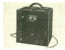
the 1E51002, the regulator measures approxi-mately  $11^{1}_{2} \ge 11^{1}_{2} \ge 10^{1}_{4}$ -in, and is fitted with carrying handles. It is rated at 95 to 135 volt input and its output is adjustable be-tween 110 and 120 volts. The load power factor range is 0.5 lagging to 0.9 leading; waveform distortion is claimed never to exceed  $3^{\circ}e_{c}$ --**superior Electric Co., Bristol, Conn.**
