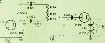
During the pulse, C106C charges to voltage E through V19. Between pulses, C106C will discharge through R84, R85 and R86, thus charging C60. After several cycles each capacitor builds up to voltage E (Fig. 8c). During pulses, voltage E on C60 adds to pulse voltage, to charge C61 and C106C through V20 to a total voltage 2E, with voltage "E" appearing across each. (Figure 8d) The output is the sum of the voltages across C61 and C106C.
