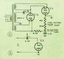
Fig. 7a shows the DuMont RA-101 voltage doubler source of high voltage for the picture tube. This differs from the usual inductive fly-back or high frequency oscilla-tor type of second anode supplies so common that a power trans-former is used, with a secondary delivering 4,400. On the negative swing of this high voltage secon-dary, C34 charges to voltage E through VII, as shown in Fig. 7b.
