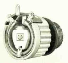
Heat dissipation properties of aluminum are used to full advantage in housing and winding core of IRC Power Rheostats, 25 and 50 watts. Type PR Rheostats operate at full rating at about half temperature rise of equivalent units. Can be operated at full power in as low as 25% of rotation without appreciable difference in temperature rise. Direct contact between rheostat and mounting panel allows rapid conduction to panel of a portion of heat dissipated. Send for Bulletin E-2.
