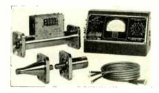
ments for measuring RF power and standing wave ratio on 51.5 ohm coaxial transmission line. A single meter reads incident power, re-flected power, not power to load, and SWR of the load. Known as the MM100 series Micromatch, these units may be used with  $15_8$  or  $7_8$  in, air line, and with RG-17/U and RG-87U coaxial cable. Full scale power ranges of 100, 1200, and 4000 watts are available.— Jones Electronics Co., 96 N. Main St., M C. Bristol, Conn.
