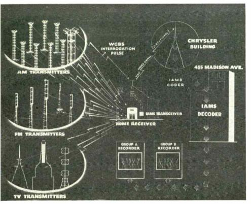
Fig. 1: Diagram illustrating overall operation of IAMS in New York City. AM listeners have not reported hearing the 7 KC interrogating pulse mixed with program material
