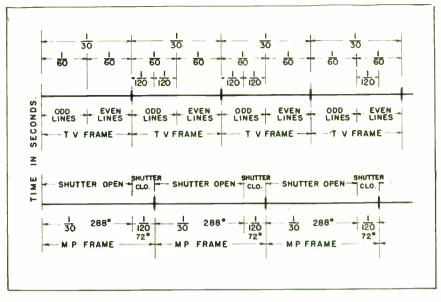
Fig. 1: Diagram illustrating the timing cycle involved in recording 30 frames per second television on motion picture film operating at 24 frames per second
