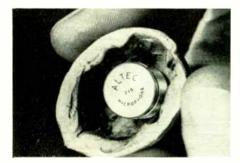
and weighing less than 1/4 ounce. size in size and weighing less than ¼ ounce. The only moving element in the microphone is an extremely small diaphragm no larger than the human eardrum, yet the sound output from this tiny apparatus is somewhat greater than from conventional large microphones. Even though the microphone is omnidirec-tional and "blast proof", more net acoustic gain before encountering feedback is claimed. -Altee Lansing Corp., 161 Sixth Ave., New York 13, N. Y.
