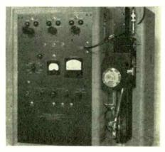
by a recently-developed microwave dielectro-meter. The instrument consists of a slotted wave guide, precision traveling probe, modu-lated klystron oscillators, probe output am-piliter, and associated power supplies. The sample to be measured is inserted ahead of a short-circuiting plug and the effect of this arrangement on the standing-wave pattern in the guide provides data for calculating the dielectric constant and loss of the material.— Central Research Laboratories, Inc., Red Wing, Mina.
