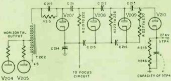
voltage. When a positive pulse appears at the top of the auto trans-former, the voltages across C211, C212, and C213 (each of value "E") add to the pulse voltage to charge the capacity between inner E") outer wall coatings of the 5TP4 to a potential of 27,000 volts, (through V210). The voltage across C214
