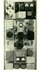
of a transmitter (illustr.), receiver. 2 dipole antennas with parabolic reflectors and R(117) coax antenna lines. The equipment includes a directly frequency-modulated GW cavity magnetron oscillator, a wide-band vidco ani-plifier and modulator, and associated regulated power supply.—Raytheon Mfg. Co., Waltham 51 Mass 54. Mass.
