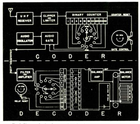
Fig. 6: Diagram showing the connections of equipment items used in relaying pulse count information from system's receiving point to graphical recorder
