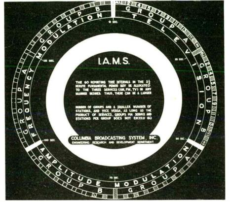
Fig. 3: Clock face for IAMS is divided into 60 reporting time intervals during one 2.5min. revolution. System can be arranged to accommodate "yes" or "no" listener vote
