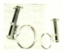
10 turns. On present swinging link assembles, it is only necessary to replace the swinging link arm with a new one, into which the link coils are plugged. This is accomplished easily by removing the pin that forms the arm hinge and inserting the new arm. -Barker & Williamson, Inc., 237 Fairfield Ave., Upper Darby, Pa.
