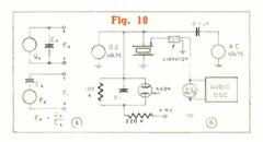
arrangement allows the sample to be charged with AC and DC potentials and further permits the sensitivity to be measured while charging with DC. The neon light is a short circuit indicator.
