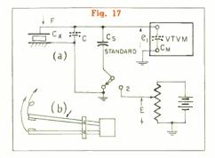
The test specimen is placed between the rubber jaws under full pressure with the switch in the (1) position. The voltmeter is shorted out momentarily to remove the induced piezoelectric charge. The up-
