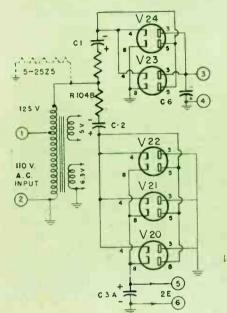
Fig. 6: In the Emerson, Model 571, five 2525 rectifier tubes are utilized. A parallel com-bination of two provides one doubler system and a parallel combination of three another
