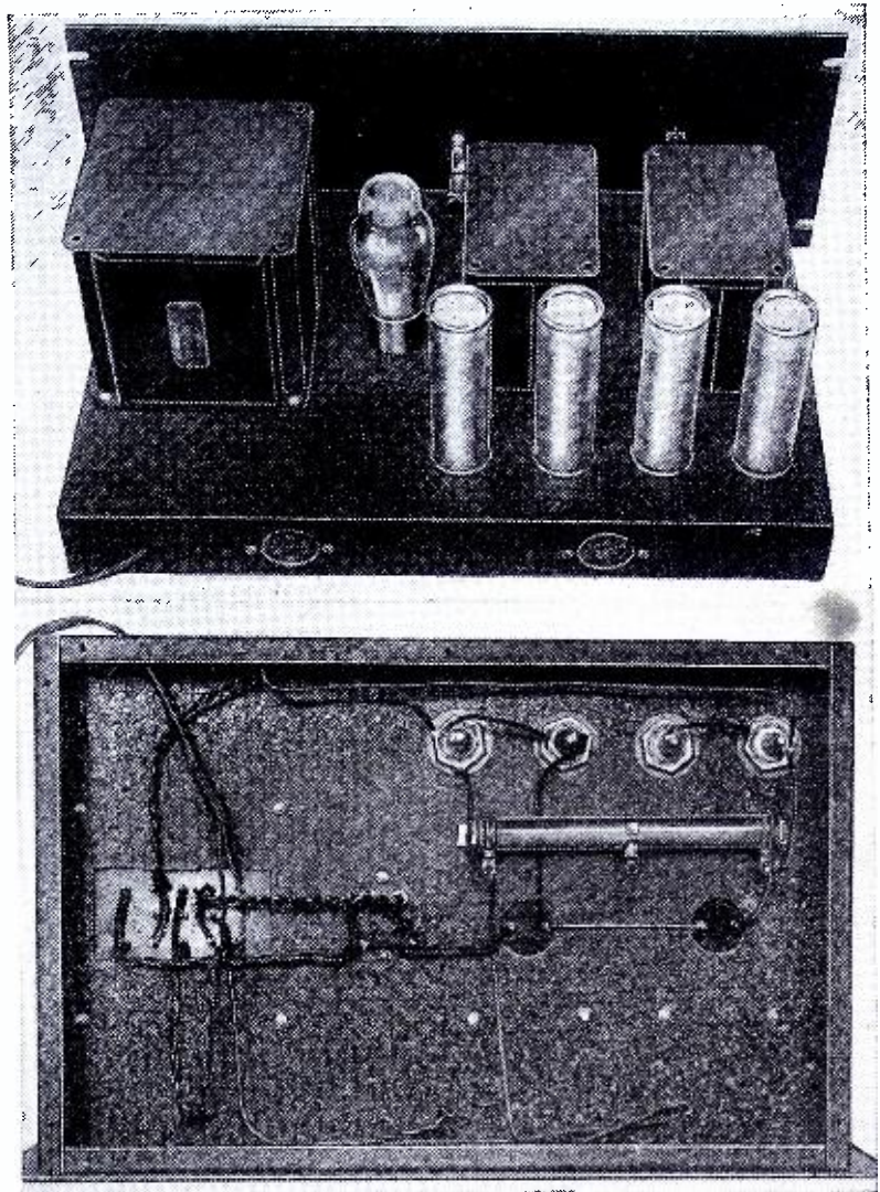
Top and bottom views of Transmitter. Diagram at Left.
