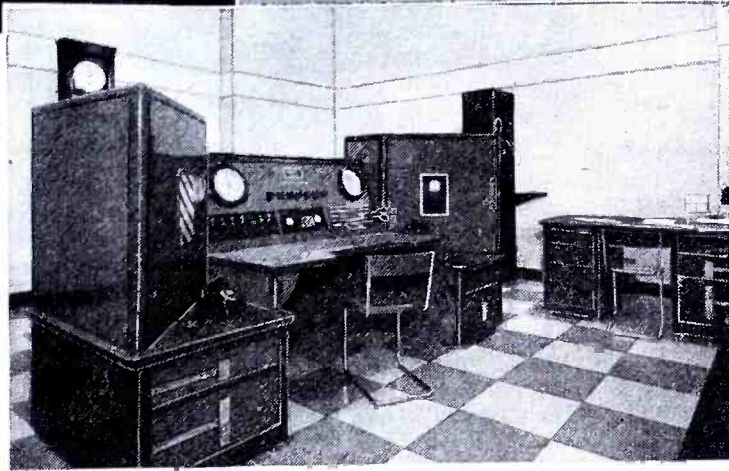
Above: All LR1, "Radio El Mundo" studios are fitted with electric clocks and also the new 3 minute clocks. Left: Control desk at Radio Station "El Mundo." At right — oscillograph and calibrating dials. Center—3 minute and secondary clocks on control panel and master clock on wall.
