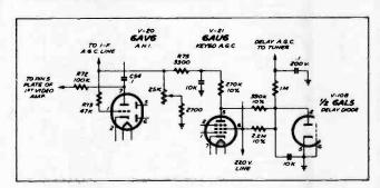
If the delayed AGC circuit is added to a 2740 chassis containing a VHF/UHF (all-channel) tuner, the following additional changes must be made:
