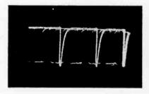
Fig. 12. Sync Separator Plate, Pin 1, 30 volts, 15,750 c.p.s.
