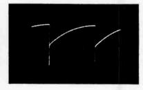
Fig. 14. Vertical-Output Grid, Pin 2, 72 volts, 60 c.p.s.
