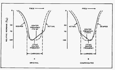
Fig. 3. Television tuner response curve, showing tracking compensation.
