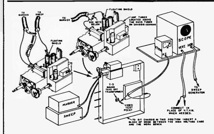
Figure 8. CONNECTIONS FOR I.F. ALIGNMENT
