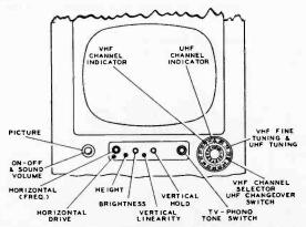
Receiver Operating Controls (UHF-VHF Models).
