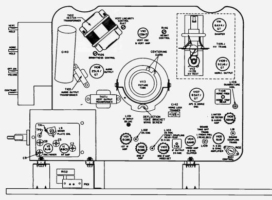
Tube and Alignment Locations 21" 1600D Chassis
