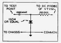
FIG. 5. Diode Detector Detail
