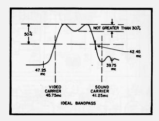
USUALLY: To set 45.75 marker, at 50% point adjust tuner IF coil.
