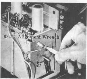
Fig. 11 Bulls-eye Tuning Adjustment
