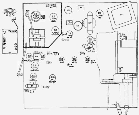
Fig. 7. Base Layout - Top View - TV-300 Chassis.
