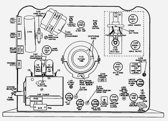
Tube and Alignment Locations 17" 1600D Chassis
