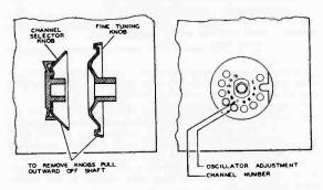
Figure 5-KRK22D R-F Oscillator Adjustments
