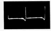
Fig. 13. Vertical-Oscillator Grid, Pin 2, .34 volts, 60 c.p.s.
