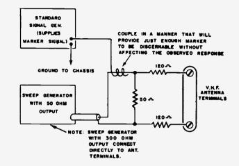
Figure 5. GENERATOR CONNECTIONS FOR TELEVISION R.F. CHANNEL ALIGNMENT.
