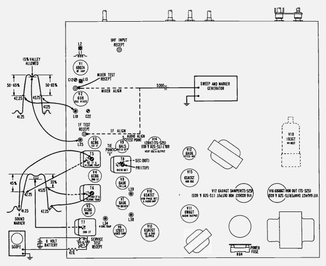
FIGURE 8. TUBE LOCATIONS & IF ALIGNMENT DETAIL
