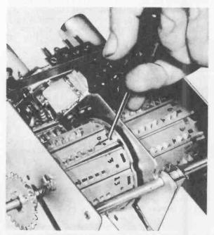
Fig. 13 Removing Channel Strips.
