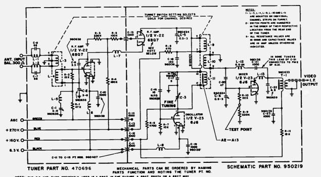
NOTE: THE R.F. AMP TUBE PRESENTLY USED IS A 6807. IN THE FUTURE A 6807, 6807A OR A 6927 MAY BE USED. THESE THREE TUBES ARE MITERCHARMSCABLE, BUY DUE TO POSSIBLE VARIATIONS IN MITERELECTROBE CAPACITIES, SEVERAL TUBES MAY MAYE TO SE TRIED FOR BEST RESULTS.
