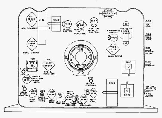
FRONT VIEW OF CHASSIS 426 (Tube & Alignment Locations)
