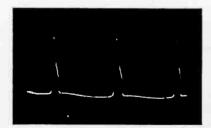
Fig. 18. Horizontal-Oscillator Cathode, Pins 3 and 8, 18 volts, 15,750 c.p.s.
