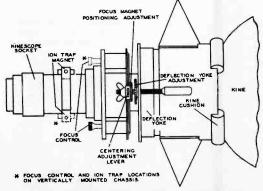
Figure 3-Yoke and Focus Magnet Adjustments
