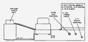
Figure 4-Rear Chassis Adjustments
