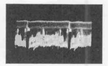
Fig. 11. Sync Separator Grid, Pin 2, 90 volts, 60 c.p.s.
