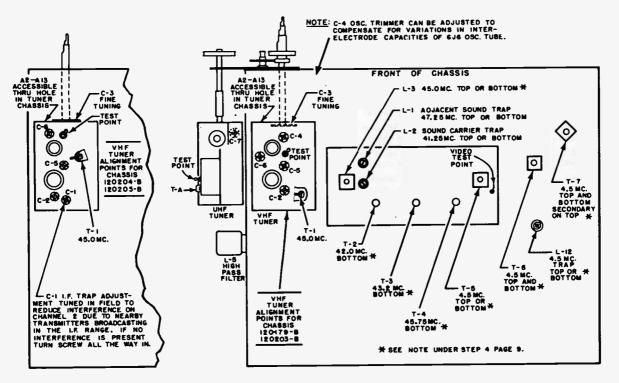
Figure 9. LOCATION OF ALIGNMENT POINTS (TOP VIEW)
