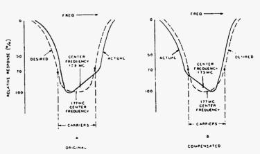
Fig. 5. Television tuner response curve, showing tracking compensation.
