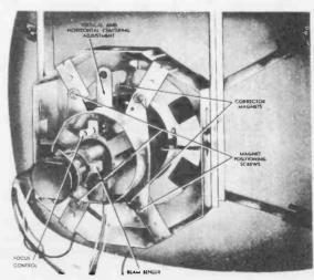
Adjustments on Neck of Picture Tube 20M21 Chassis
