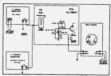
FIG. 3. IF ALIGNMENT BLOCK DIAGRAM
