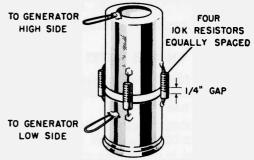
Figure 7. Special Tube Shield for IF Alignment and IF Response Curve Check.
