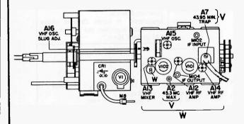
Figure 31. Top View of TV Tuner Showing Adjustment Locations.
