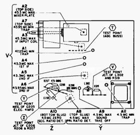
Figure 32. Bottom View of 19T1, 19W1, and 19W1A Chassis Showing Test Point Connections and IF Alignment Data.
