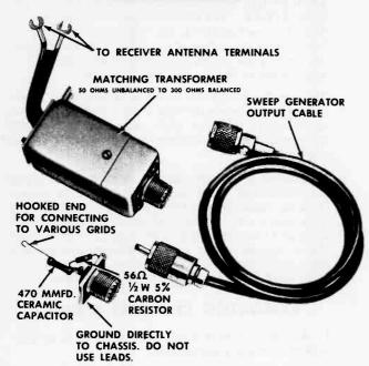
Fig. 14 IF-RF Alignment Fixtures
