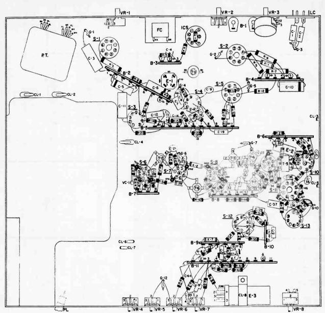
Fig. 22. Wiring Diagram, Bottom View -- TV-300.
