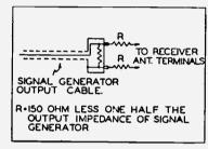
FIG. 4. Dummy Antenna Detail
