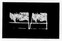
Fig. 9. Composite Signal, Pin 2 of 12BY7, 6 volts, 15,750 c.p.s.
