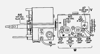
Figure 38. Top of Tuners, Showing VHF Adjustment Locations.
