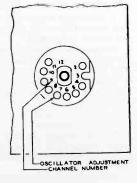
Figure 6-KRK30 VHF R-F Oscillator Adjustment
