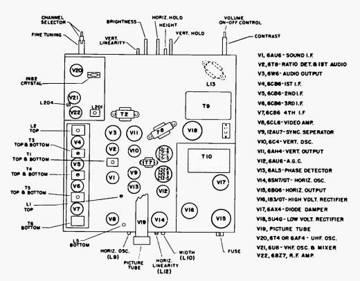
Fig. 2. Top View -- All chassis except 528.300, 300-1, 300-2 and 300-3
