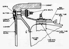
Fig. 10. Detail of Picture Tube Mount (Models 17T15, 21T10-T11-T12)
