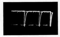
Fig. 12. Sync Separator Plate, Pin 5, 41 volts, 15,750 c.p.s.
