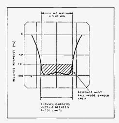
Fig. 4. Television tuner response curve, showing bandpass limits.
