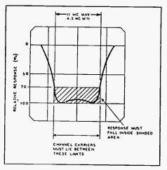
Fig. 2. Television tuner response curve, showing bandpass limits.
