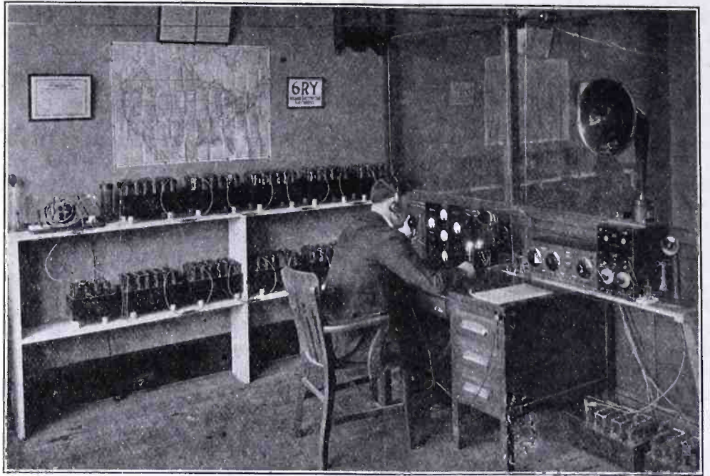
Radio Station 6RY, Employing Storage Batteries to Give 500 Volt Plate Potential
