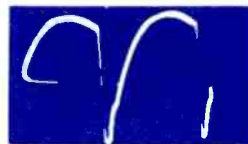
⑪ SR201 CATHODE JUNCTION HORIZONTAL PHASE DETECTOR HORIZONTAL RATE 9V P-P
