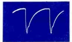
⑭ V101 PIN 9 HORIZONTAL OUTPUT GRID HORIZONTAL RATE 85V P-P
