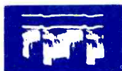
② V205 PIN 9 VIDEO OUTPUT PLATE VERTICAL RATE 70V P-P
