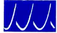
11 TP201 VERTICAL OUTPUT CATHODE VERTICAL RATE 15V P-P
