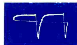
④ V201 PIN 1 SYNC PLATE HORIZONTAL RATE 48V P-P
