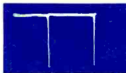
⑩ V105 PIN 2 PICTURE TUBE GRID VERTICAL RATE 62V P-P
