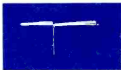
⑨ PW-200, TERMINAL "L" VERTICAL OUTPUT TRANSFORMER VERTICAL RATE 350V P-P
