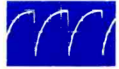
12 V105-2, 6 HORIZONTAL OUTPUT GRID HORIZONTAL RATE 235V P-P
