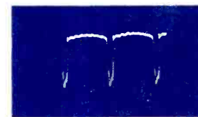
15 V105 PIN 3 KINESCOPE 1ST ANODE HORIZONTAL RATE 40V P-P
