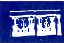
⑦ V205B PIN 9 VIDEO AMPLIFIER PLATE VERTICAL RATE 110V P-P
