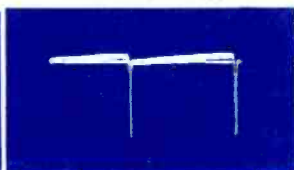
⑨ PW-200, TERMINAL "L" VERTICAL OUTPUT TRANSFORMER VERTICAL RATE 150V P-P
