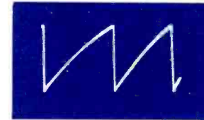
6 V206A PIN 2 VERTICAL OUTPUT GRID VERTICAL RATE 28V P-P
