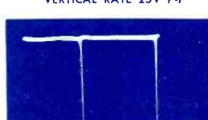
⑩ V105 PIN 1 PICTURE TUBE GRID VERTICAL RATE 110V P-P
