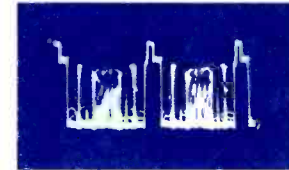
8 V205B PIN 9 VIDEO AMPLIFIER PLATE HORIZONTAL RATE 110V P-P
