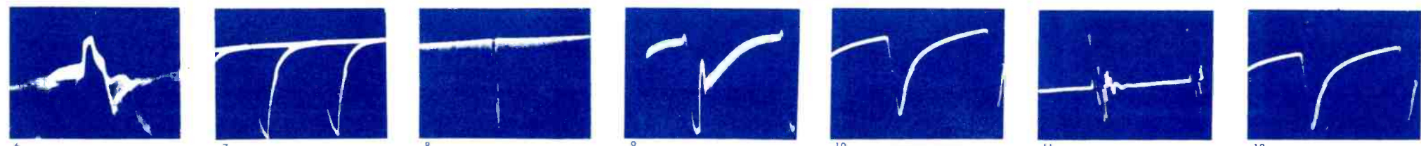
6 TP501 60V P-P (HORIZ.) SYNC SEPARATOR GRID 7 JUNCTION R516 & R545 70V P-P (HORIZ.) SYNC SEPARATOR PLATE 8 JUNCTION R516 & R545 80V P-P (VERT.) SYNC SEPARATOR PLATE 9 COMMON CATHODE 13V P-P (HORIZ.) HORIZ. PHASE DETECTOR 10 V503-9 (C515) 300V P-P (HORIZ.) HORIZ. OSCILLATOR GRID 11 TP503 300V P-P HORIZ. HORIZ. OSCILLATOR COIL 12 PW500W 300V P-P (HORIZ.) HORIZONTAL DRIVE
