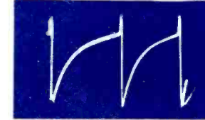
5 V206B PIN 9 VERTICAL OSCILLATOR GRID VERTICAL RATE 180V P-P
