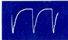
2 V101 PINS 2 & 6 HORIZONTAL OUTPUT GRID HORIZONTAL RATE 130V P-P
