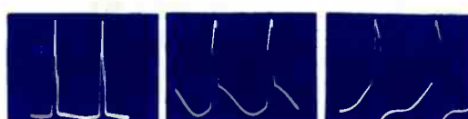
16 9 Volts p/p, 15,750 cps 17 34 Volts p/p, 15,750 cps 18 29 Volts p/p, 15,750 cps
