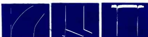
10 40 Volts p/p, 60 cps 11 1300 Volts p/p total, 120 Volts p/p, sawtooth, 60 cps 12 60 Volts p/p, 60 cps
