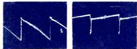
⑩ 1.5V P-P (V) BASE T34 ⑪ 50V P-P (V) COLLECTOR T34
