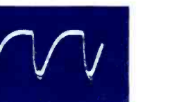
⑱ SR201 ANODE HORIZONTAL PHASE DETECTOR HORIZONTAL RATE 15V P-P
