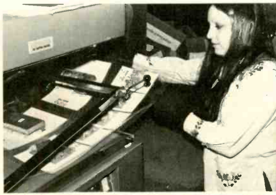
Fig. 5—Polyethylene "skin" packaging protects the rebuilt modules against dirt, dust and damage.
