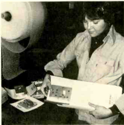
Fig. 6—A skin-packaged rebuilt module is inserted into the shipping container, stamped with the original manufacturer's type and number.
