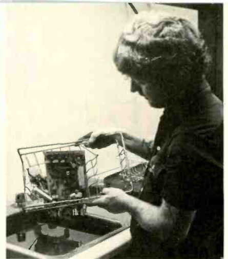
Fig. 2—In the initial step of the module rebuilding process, incoming modules are thoroughly cleaned.
