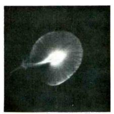
Fig. 8—An out-of-sync chroma reference oscillator causes rapid rotation of the vector pattern.
