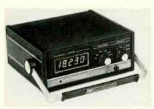
tion is 500 V DC or peak AC with CMRR of 120 dB at DC, greater than 100 dB at 50 and 60 Hz. The unit is equipped with its own internal NiCd battery module and recharger. It operates as a conventional benchmounting laboratory DMM. Operated continuously on AC line power, the batteries remain on charge whether the instrument is off or on. When not line connected, it automatically operates from its batteries for at least six hours. The multimeter measures 8½ inches wide by 3½ inches high by 7½
