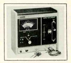
ment. The base (or gate) lead is automatically identified by the color in the small window on the front panel; collector and emitter leads are color identifiable in the same window. With one flip of a lever switch, you can determine if any PNP or NPN device is good, and you also get automatic set-up of lead connections for further testing. The unit measures 8 inches by 7 inches by 3½ inches and is priced at \$150.
