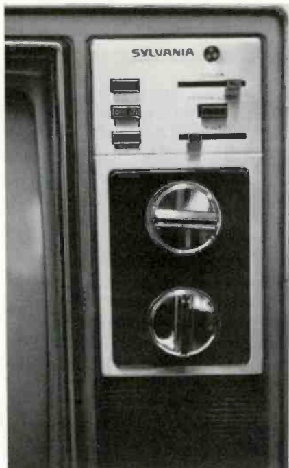
Pushbutton switches are employed to raise or lower the volume, turn the TV-set ON or OFF, or to engage the AFC. The Perma-Lock circuits are engaged by pushing a button, which lights up when the set is properly tuned. Slide type COLOR and TINT controls are also used.
