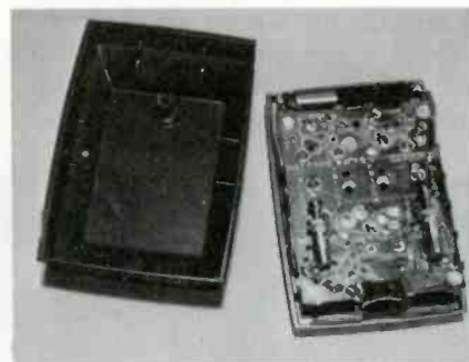
The hand-held remote transmitter consists of a transistorized oscillator with discrete frequency selection buttons for performing the various functions.
