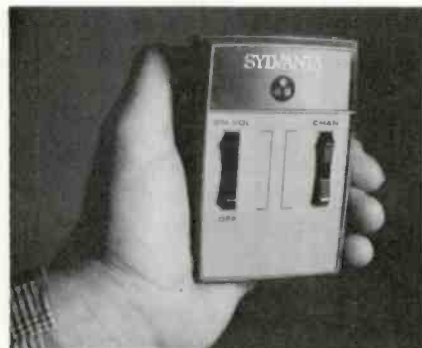
The small simplified transmitter is powered by a 1.5v battery. It has three control functions: ON/VOLUME UP, OFF/VOLUME DOWN, and CHANNEL SELECTION.
