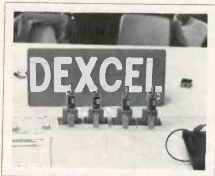
Fig. 8 Four Dexcel LNA's. Each has 33dB, minimum gain.
