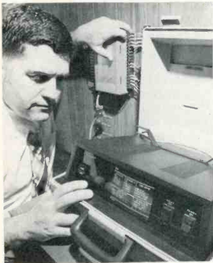
Fig. 2—An example of types of test gear field service technicians of the future will be working with is this portable, microprocessor controlled diagnostic tool. For use in troubleshooting Honeywell's heat pump control system, the field technician simply connects to the unit under test and automatic "error" messages display location and type of trouble.
