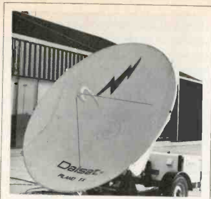
Fig. 6 Dalsat uses an Andrews dish with the feed horn and wave guide rotatable from its base.
