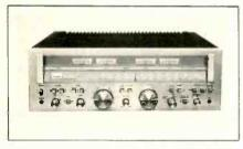
to 200kHz (+0-3dB). The G-7500 is rated at 90 watts RMS per channel, both channels driven into 8 ohms from 20-20,000Hz with no more than 0.025% total harmonic distortion. The slew rate is 60V/µsec and the rise time is 1.4µsec. The suggested retail price is \$620.
