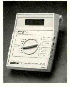
changing is automatic. Measurement ranges are dc and ac volts from .1mV to 1000V, dc and ac current from .001mA to 10A and resistance from .1 ohm to 19.99 megohms. The accessories include a hold probe which will hold a reading if the operator's eyes have to remain on the test point during measurement, a light meter attachment, HF and VHF RF probes, a 50KV high voltage probe, an ac clamp on amp-meter and a carrying case.
