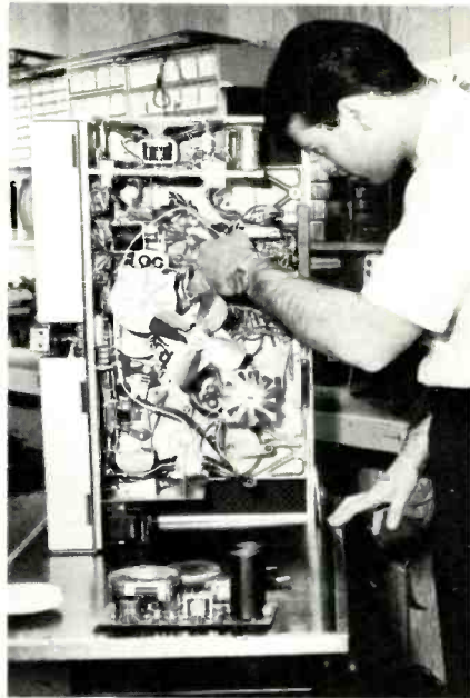
Clark Trimble, one of Tri-Video's six technicians, checks drive assembly on video tape recorder in for service.
