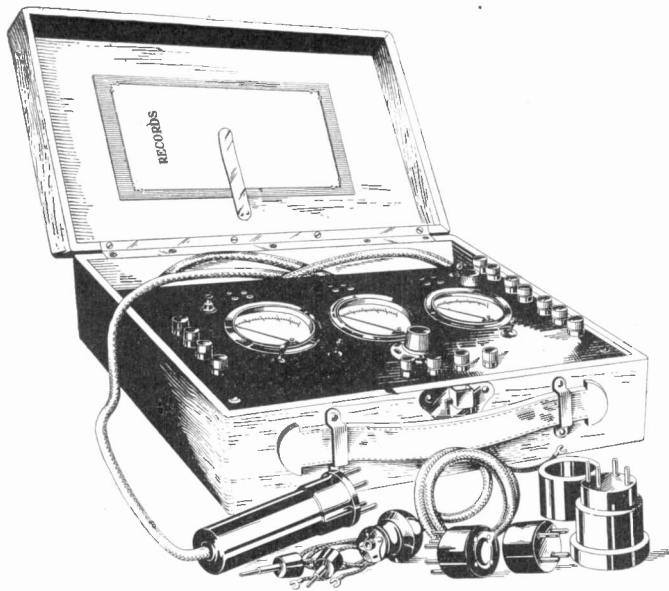
Artists conception of completed A.C.-D.C. set tester. Space may be left in the rear of the carrying case for wires, cables and the various adaptors as shown.
