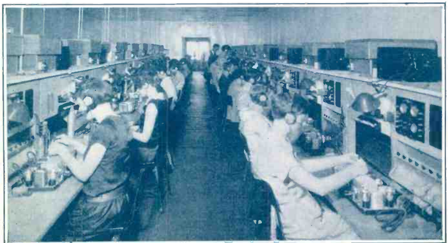
The "English roundhouse" an unique booth where 3,000 receiving sets are balanced and tested each day at the plant of the Crosley Radio Corporation, Cincinnati, O.
