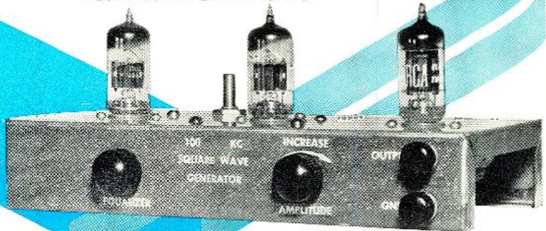
Fig. 1. Over-all view of square-wave generator built by the author at relatively low cost. A small cabinet or metal box can be used instead of open chassis.
