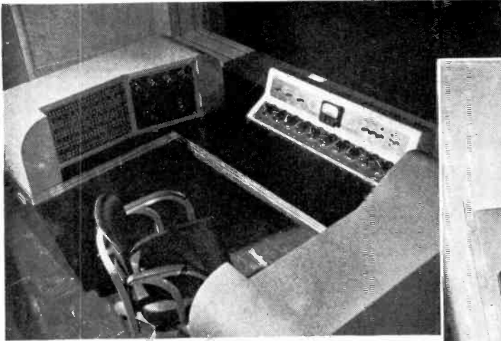
Custom-built speech input console. Mutual Don Lee's new Hollywood headquarters include four large auditorium studios, each 170,000 cubic feet in volume and seating 350 people. All of these four studios have Western Electric control consoles located in the control booths which are at left of the stages.
