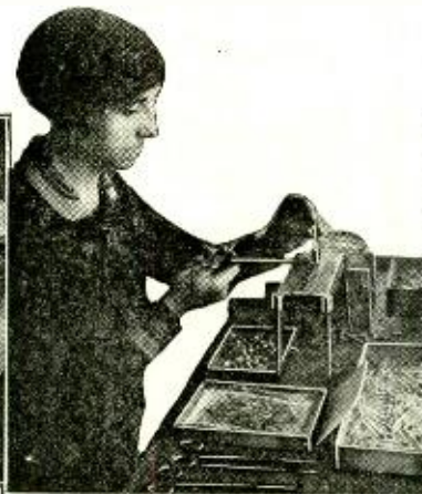
Here an operator is shown holding the cap and tube in a special pair of pliers and soldering the coated filament in place.
