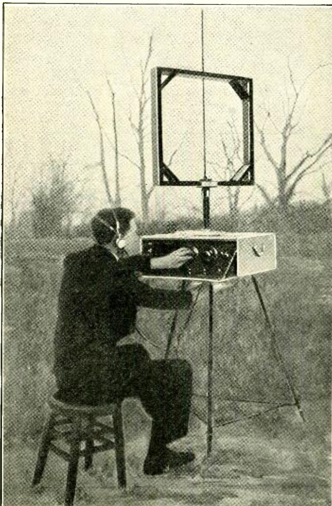
Fig. 1. The portable superheterodyne erected on its tripod with the loop in position for receiving.
